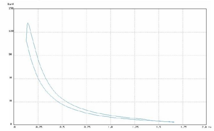
The pressure/volume diagram displays the classical  $p \sim V$  diagram used in thermodynamic calculations to measure the power produced within a cylinder. The x -axis displays the swept volume of the piston.
