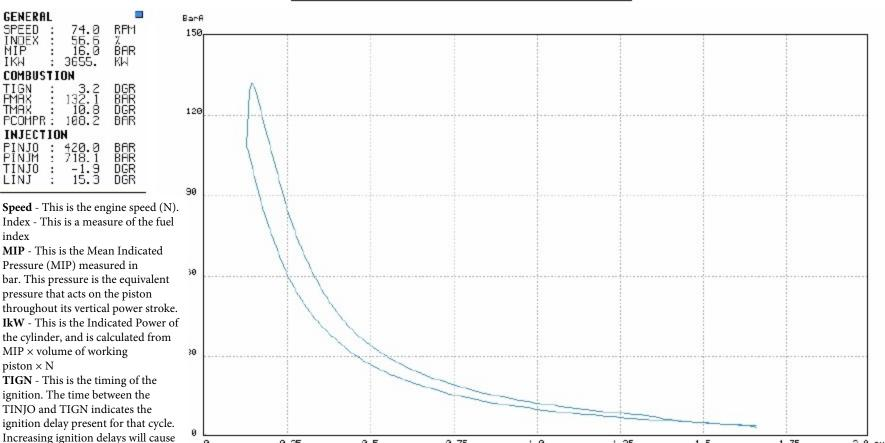
**TMAX** - This is the position of the maximum temperature during the working cycle.
