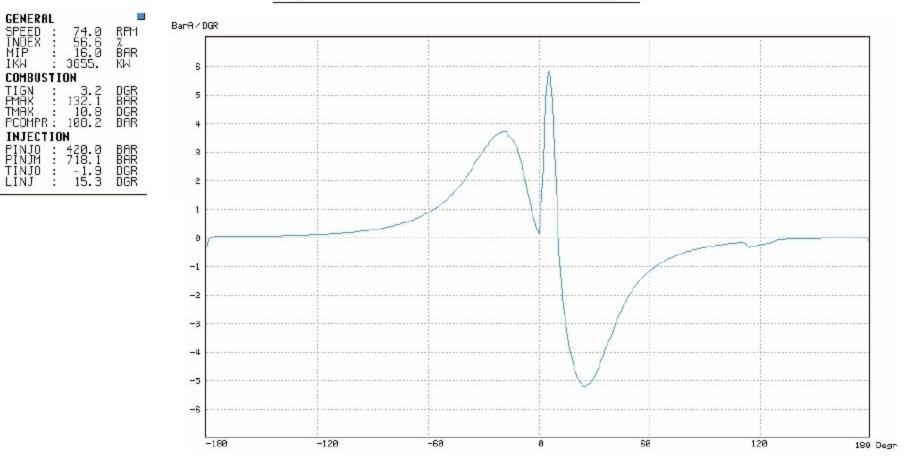
The delta pressure / angle or pressure derivative graph is used to provide additional information about the combustion process by displaying the rate at which the pressure changes within the combustion chamber.
