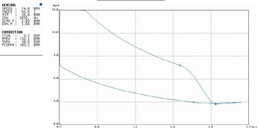
The weak spring diagram displays the scavenging process of the cylinder. The graphical display identifies the position of the opening of the exhaust valve, the opening and closing of the scavenge ports (same point before and after bottom dead centre), and the closing of the exhaust valve.
