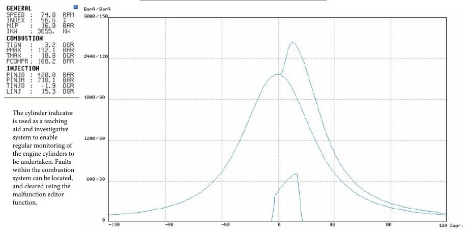
There are four different displays that can be selected to indicate the cylinder pressure conditions, namely pressure/angle (also called a draw card or out of phase diagram), pressure/volume (also called a power card, or in-phase diagram), the weak spring diagram, and the delta pressure/angle diagram. Each diagram can be used to illustrate differing combustion traits.
