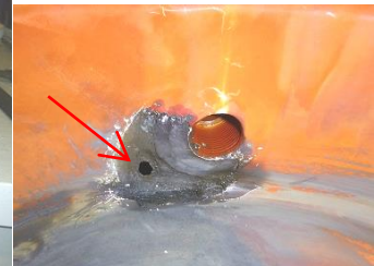
Photo 2. Peeling and pinhole of the bottom cover
