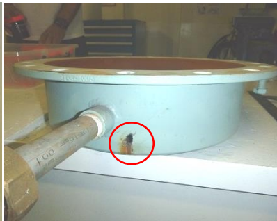
Photo 2. Peeling and pinhole of the bottom cover
