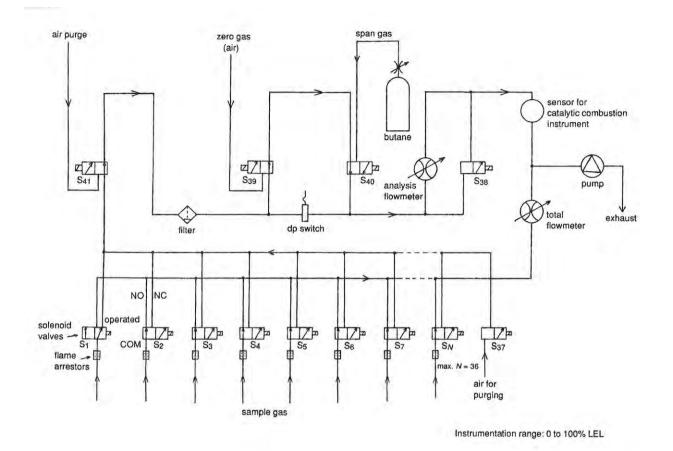
Figure 2.2.1.10(A) FLOW DIAGRAM OF A FIXED GAS – DETECTING SYSTEM
