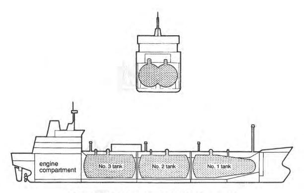
A semi-pressurized/fully refrigerated LPG/NH3 carrier
