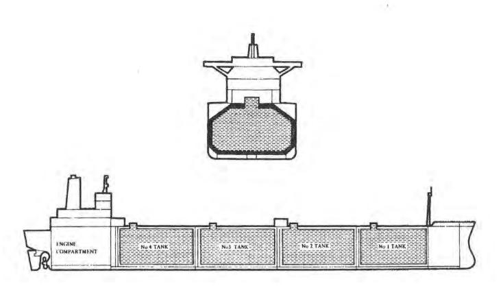
Figure 1.1 (H) A FULLY REFRIGERATED LPG CARRIER
