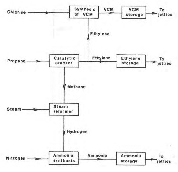
Figure 3.1.10 FLOW DIAGRAM FOR TYPICAL PRODUCTION OF CHEMICAL GASES
