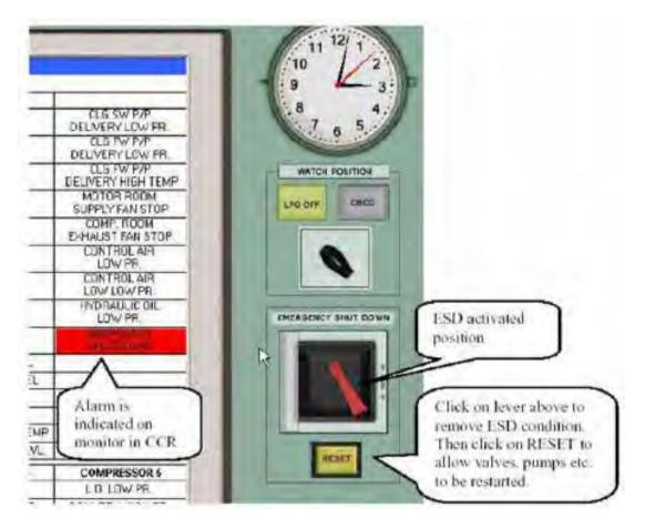
Figure 2.4 (A) ESD Reset LIQUID CARGO HANDLING SIMULATOR – LPG
