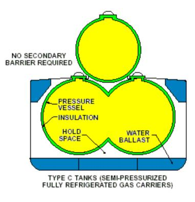
Figure 1.1.8 (D) SEMI PRESSURISED LPG SHIP
