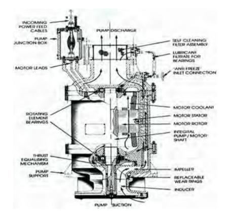
Figure 2.3(I) SUBMERGED MOTOR PUMP FOR LPG
