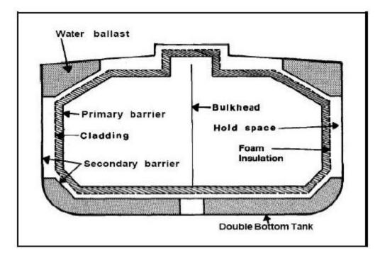
Figure 1.1.8 (A) CONTAINMENT SYSTEM LPG TANK
