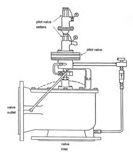
Figure 2.2.2(A) A CARGO TANK SAFETY RELIEF VALVE
