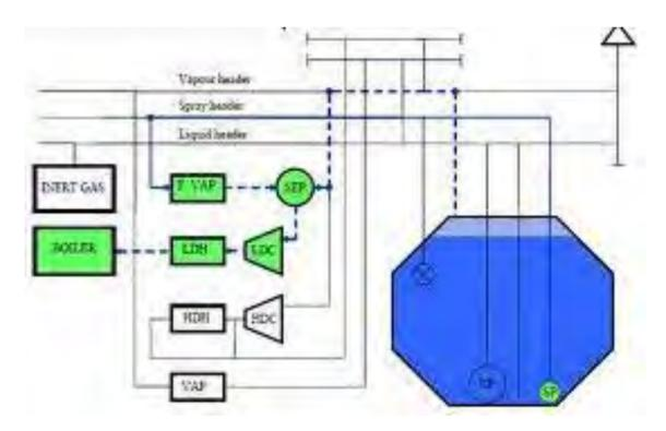
Figure 2.2.3 (D) LOADED VOYAGE WITH FORCED VAPORIZER
