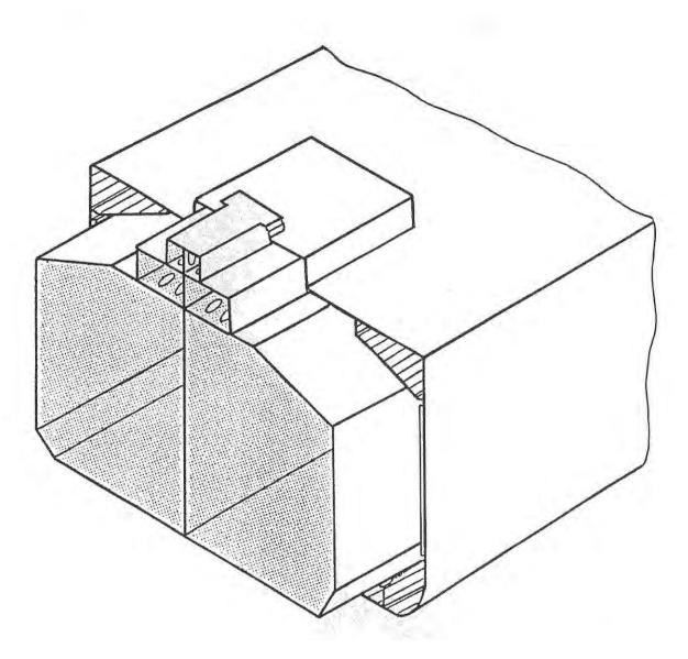
Figure 1.1.8 (K) AN INDEPENDENT TANK OF TYPE A (FOR LPG)
