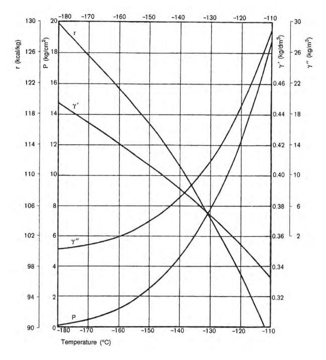
Figure 7.1.2 ICS CARGO DATA SHEET FOR METHANE
