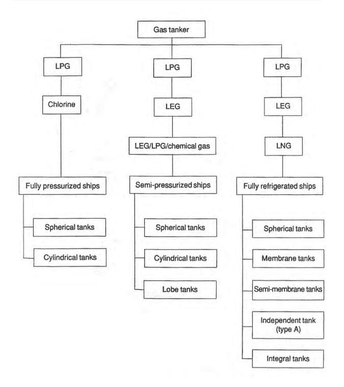
Figure 1.1 (I) BLOCK DIAGRAM DESCRIBING GAS TANKER TYPES AND THE RELATIONSHIP BETWEEN THE CARGO CARRIED, CARRIAGE CONDITION AND THE CARGO – CONTAINEMENT SYSTEM NORMALLY USED.
