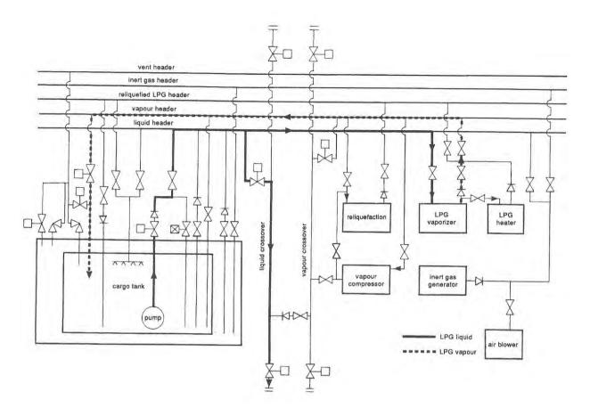
Figure 2.3 (B) CARGO DISCHARGING, WITHOUT VAPOUR RETURN
