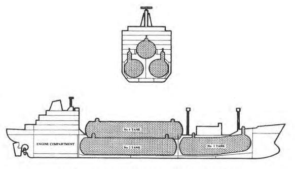
A semi-pressurized/fully refrigerated LPG/NH3 carrier
