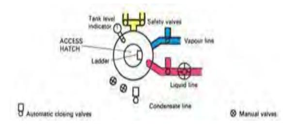
Figure 1.2 (B) TANK DOME PENETRATION
