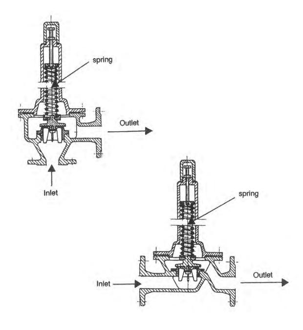
Figure 2.2.2 (C) SPRING – LOADED RELIEF VALVES
