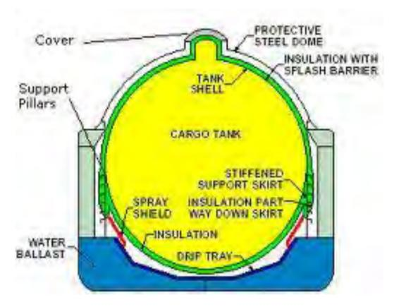
Figure 1.1.8 (E) SELF-SUPPORTING SPHERICAL TYPE B TANK
