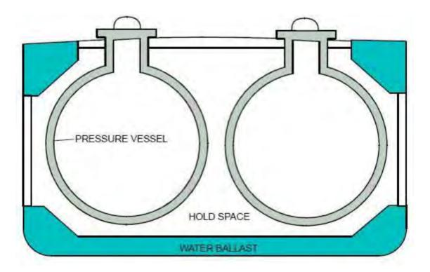
Figure 1.1.8 (B) FULLY PRESSURED CONTAINMENT SYSTEM
