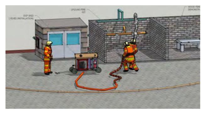
Figure 2: LPG / LNG fire pit view and demonstration of extinguishing of fire by using fixed DCP system
