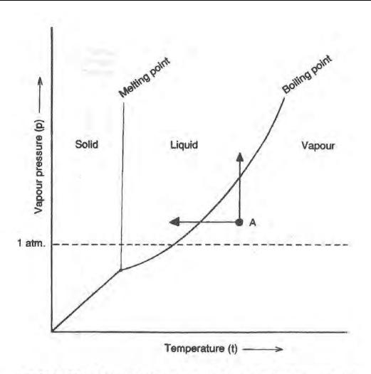
.... a gas (A) can be liquefied by removal of heat and/or pressurizing ....
