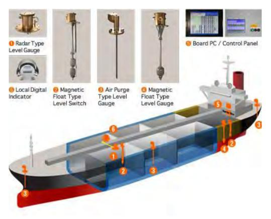
Figure 2.2.1.4 CARGO HANDLING EQUIPMENT- GAUGES
