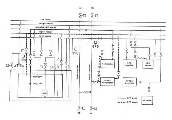
Figure 2.5(I) CARGO CONDITIONING DURING LOADED PASSAGE
