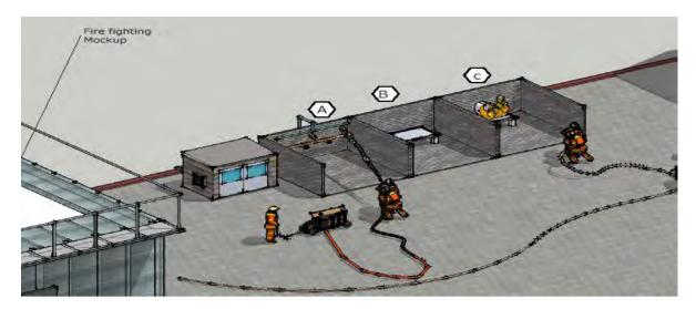
Section A, B and C for Gas, Wood and Oil fire demonstration
