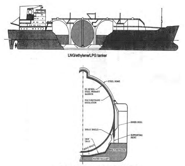
Independent self-supporting spherical tank (type B)
