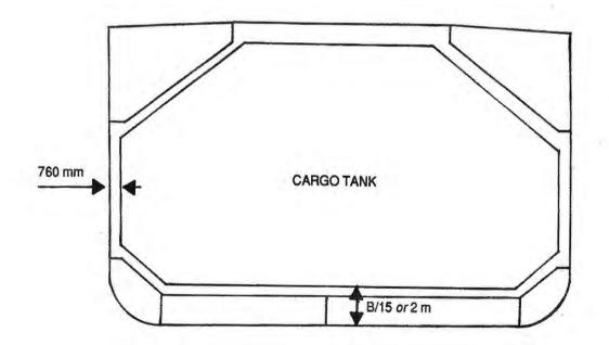
Figure 1.1.8(J) LOCATION OF CARGO TANKS IN SHIPS OF TYPES 2G, 2PG AND 3G
