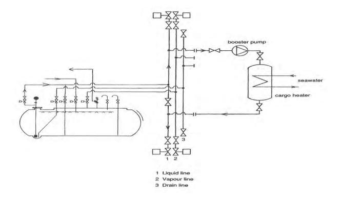
Figure 2.2.3(C) SCHEMATIC DIAGRAM OF A CARGO HEATER ARRANGEMENT
