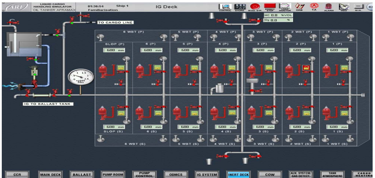
Oil Tanker Fig 5: IG and Venting arrangements of an oil tanker Simulator Screen
