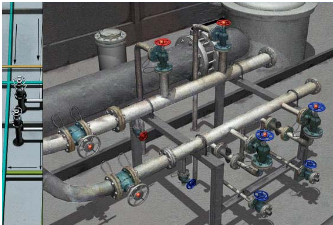
Chemical Simulator Fig 6: Tank Heating arrangements on a Chemical Tankers main deck
