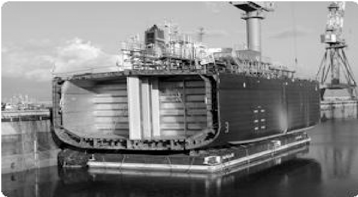
Fig. 1.2: Sophisticated Parcel Chemical Tanker with Transverse and Vertically corrugated Stainless Steel Bulkheads
