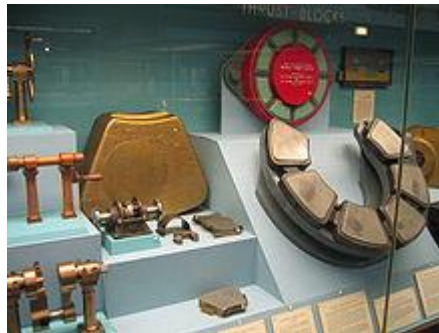
Image 6. 3 Thrust block (Mitchell type) ( Wikipedia )
