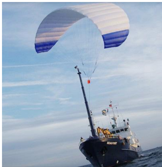
Image 9. 1 Propulsion with wind kite
