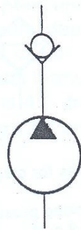
Check valve prevents the load from causing reversal pump drive when it is being lowered
