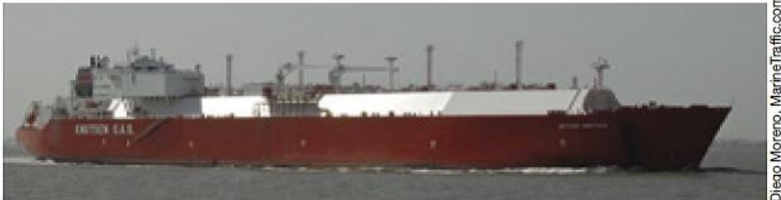
B. S/S Sestao-Knutsen can deliver its payload of nearly 1 million bbl of LNG in less than 16 hours
