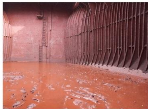
Figure : Iron ore fines after transportation in the hold of a bulk carrier (Crouch & Aamlid, 2009).
