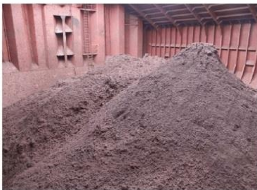
Figure : Iron ore fines after loading in the hold of a bulk carrier (Crouch & Aamlid, 2009).
