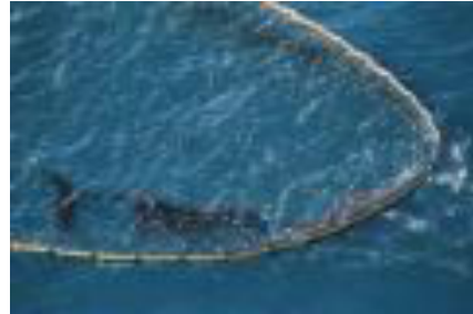
Picture 4- A boom trapping oil on the surface of the ocean
