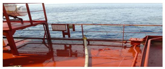
Water cannons – These are designed to deliver water in a vertical sweeping arc thus protecting a greater part of the hull. Many of these have been developed from tank cleaning machines.
