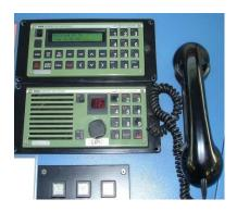
Marine VHF radio equipment is installed on all large ships and most seagoing small craft. It is also used, with slightly different regulation, on rivers and lakes. It is used for a wide variety of purposes, including summoning rescue services and communicating with harbors, locks, bridges and marinas.
