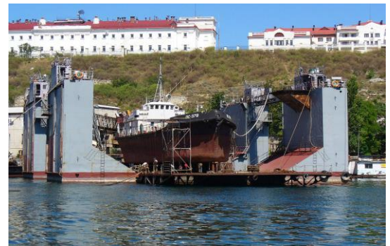
Picture 5-Floating drydocking
