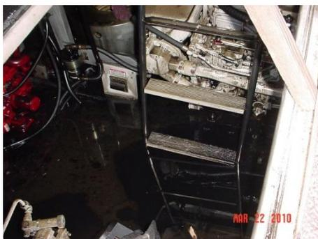
Engine room flooding as the name indicates, means filling up of the engine room space with water. Engine room flooding can affect the water tight integrity of ship. In this article we will find out what are the main reasons for engine room flooding what has to be done in case of engine room flooding.
