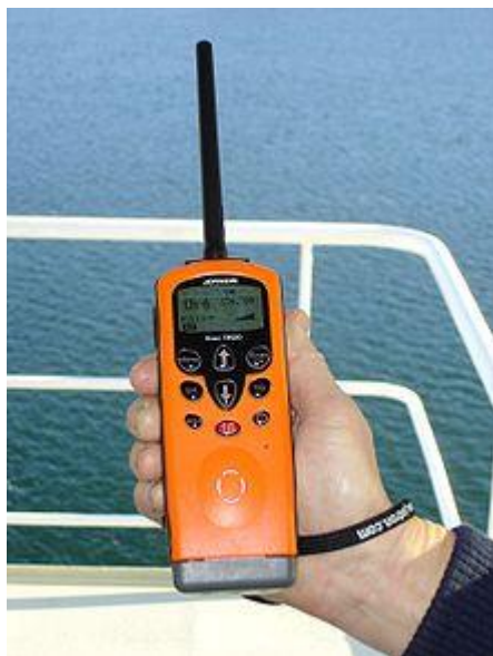
A standard handheld maritime VHF, mandatory on larger seagoing vessels under the GMDSS rules ( https://en.wikipedia.org/wiki/Marine_VHF_radio )
