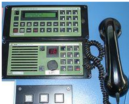
A VHF set and a VHF channel 70 DSC set, the DSC on top ( https://en.wikipedia.org/wiki/Marine_VHF_radio )
