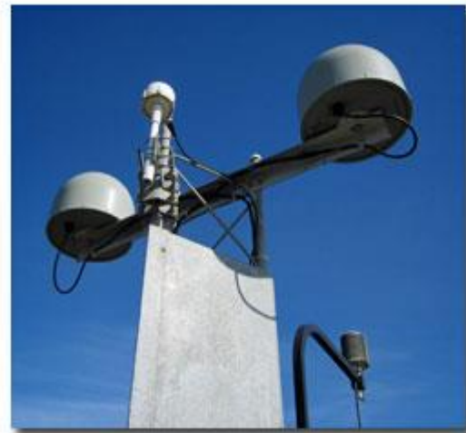
Picture 4.5 DGPS reference station antenna
