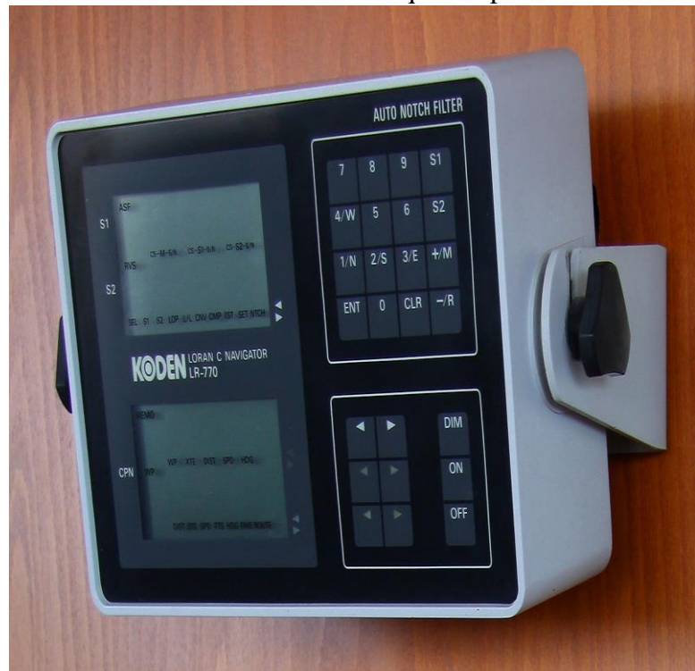
Picture 4.3 Loran-C repeater
