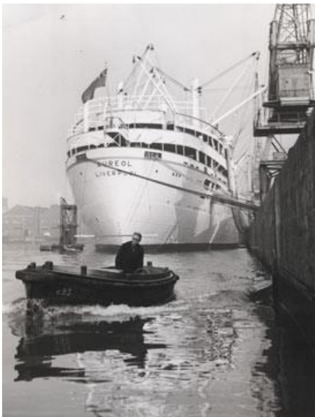
Ethel worked as a gig-boat around the docks of Liverpool and the Wirral. Gig-boats transported mooring ropes from deep-sea ships to the quaysides and would also transfer people and luggage between ships and land.
