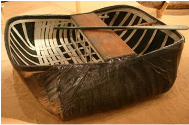
Coracles like this were used extensively for fishing on the River Dee as the flexible, lightweight and flat bottomed boats were ideally suited to the strong currents and rocky bed of the river.
