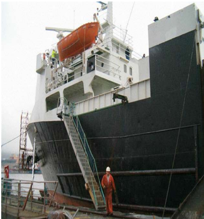
Means of access incorrectly rigged
