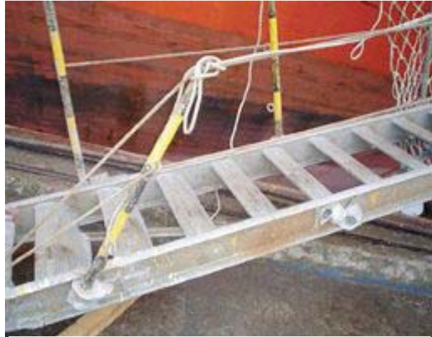
Gangway in need of maintenance
