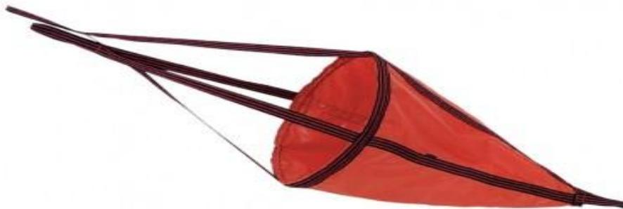
You make this adjustment by opening or closing the sea anchor's apex. When open, the sea anchor acts as a drag that keeps you in the general area. When closed, it forms a pocket for the current to strike and propels the raft in the current's direction. Additionally, adjust the sea anchor so that when the raft is on the wave's crest, the sea anchor is in the wave's trough. Wrap the sea anchor rope with cloth to prevent its chafing the raft.
