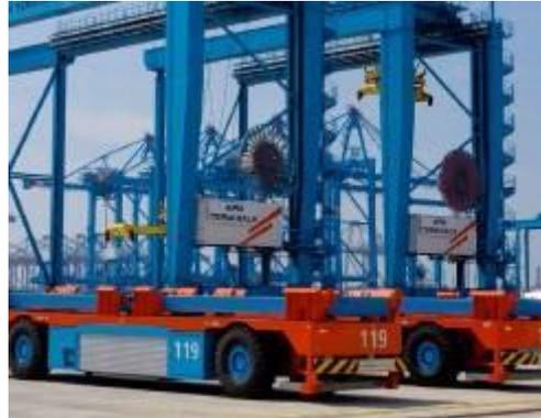
The Battery Lift-AGV allows APM Terminals to achieve higher levels of performance while minimizing environmental impact. With diesel-electric Lift-AGVs, the diesel engine produces CO<sub>2</sub>/NO<sub>x</sub>/particulate emissions at the terminal. By removing the diesel engines, APM Terminals has removed all local emissions (CO<sub>2</sub> / NO<sub>x</sub> / particulate matter) at the terminal, as well as eliminating diesel engine noise.
