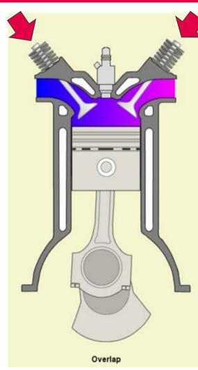
Exhaust and Inlet Valve Overlap
