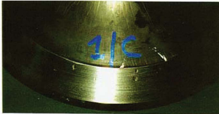
Photo 5: Acceptable seat condition after grinding
