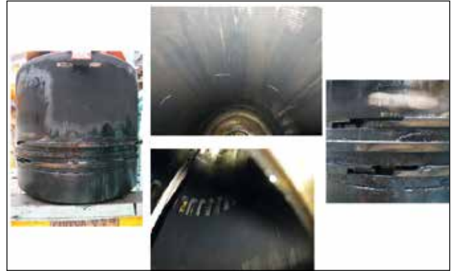
Fig. 45: T/C cut-out test and black carbon deposits
