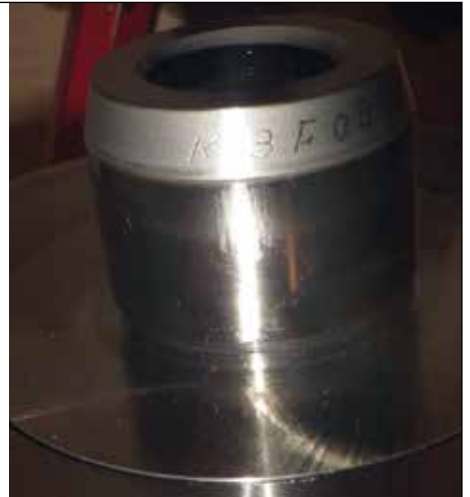
No cavitations found directly on damper
