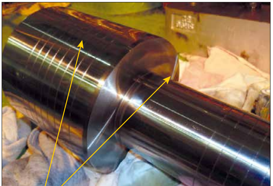
Perfect running surface, no cavitation found in grooves
