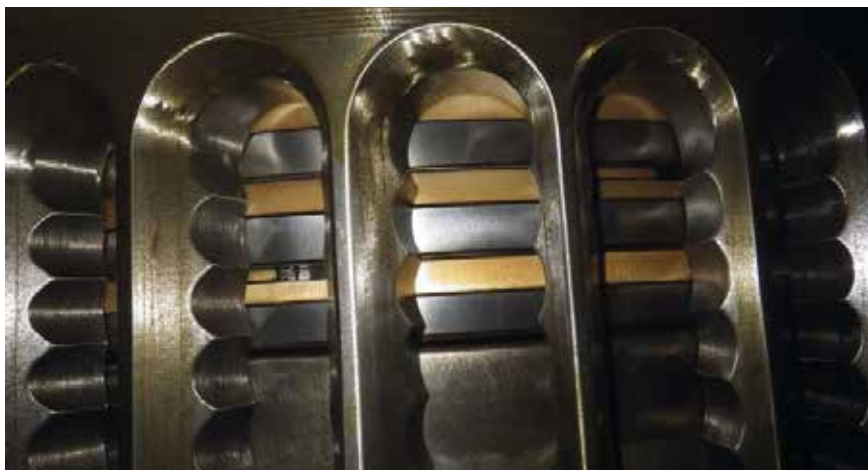
Fig. 47: T/C cut-out test with emergency bypass installed. No black carbon deposits visible.
