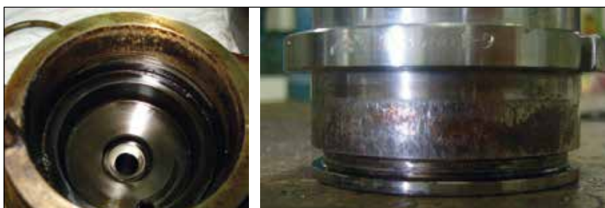
1: Fretting valve head/thrust piece 2: Fretting valve holder/valve head
