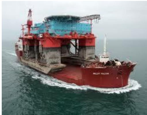
Heavy lift ships are used for very heavy cargo they are submersible.
