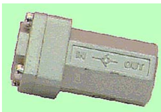
Fig. 13 (a) Non-return valve (b) Cross section
