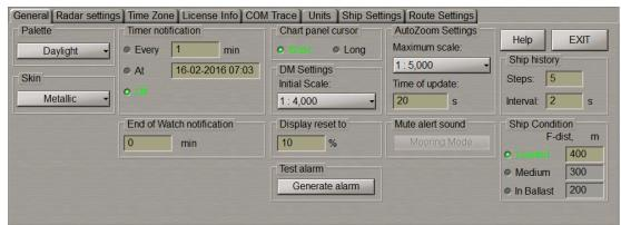
In AutoZoom Settings group from the drop-down list, select the maximum scale as the ship is passing the current WPT on Dual panel. In Time of update input window, set the DTW analysis interval.
