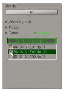
From the drop-down list select the necessary voyage(s) and check the checkbox(es) next to its/their name(s). While printing out the Ship Logbook, it is also possible to filter events by their names. To do this, press the Filter button.
