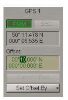
The ship symbol will move to the corrected coordinates, the coordinate offset will be displayed in **Offset** window, whilst position window will show corrected coordinates from position source.
