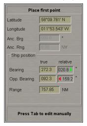
Set the cursor in the start point coordinates by moving the trackball/mouse, using the data in **Place First Point** window, and press the left trackball/mouse button.
