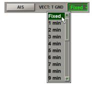
Select the required vector length (see document *Multi-Functional Display (v. 3.00.340). Functional Description*, *Chapter 3*, section *Own Ship Motion Data*, paragraph *Own Ship Motion Vectors*) from the list, which will open up and press the left trackball button.
