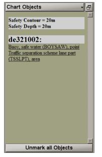
The display shows all the dangers which happen to be within the anchorage zone (Swing Circle). The following chart objects should be considered as dangerous during the anchorage:
