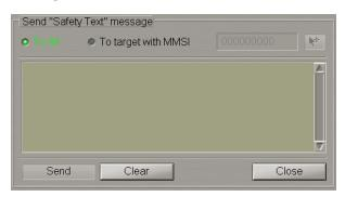
Set the identifier of the addressee of the message to be sent. To transmit a message to all the ships in the radio coverage area, check **To All** checkbox.
