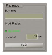
Press Find button. Position the graphic cursor, which will appear, on the point within the Chart panel which will be the centre of the area coverage circle.
