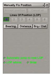
**Manually Fix Position** display is intended for constructing the ship line of position (LOP) by measuring bearing and/or range to one or more visible objects whose coordinates are known in advance (or the object can be uniquely identified on the chart).
