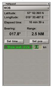
The **Show seek circle** button is enabled by default. Use the input box to the right of the button to enter the seek circle expansion rate different from 0.
