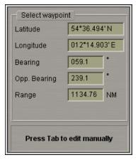
Press the left trackball/mouse button: the marker will acquire the WPT and change own form. Position the marker in the new reference point within the displayed Chart Panel.
