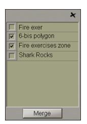
In the window which will open up, check the checkboxes next to the maps which should be merged.
