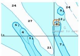
Press the left trackball button: "Deleted object" attribute is removed, and the object is highlighted in accordance with the previously made settings.
