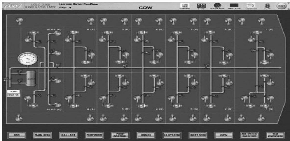
Figure 1 (U) Crude oil Washing Layout
