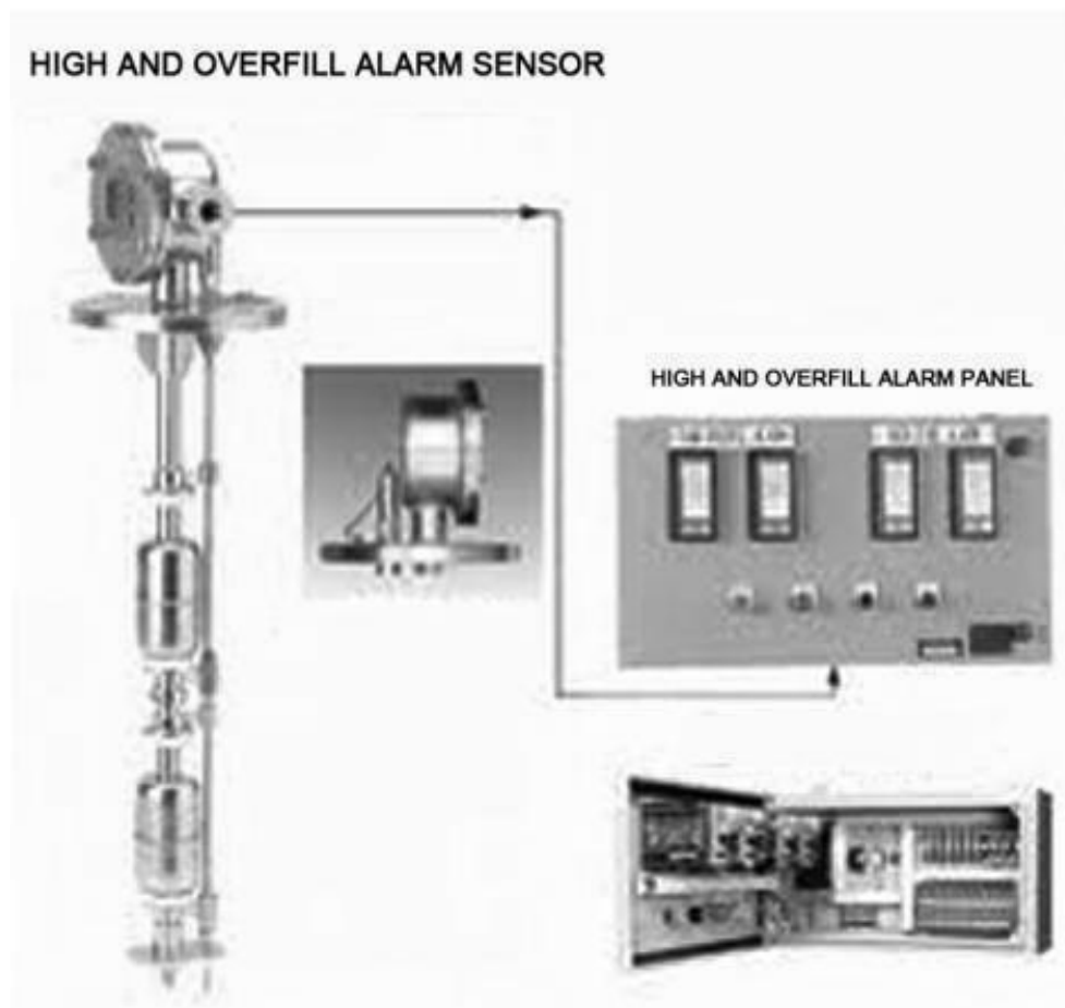
Fig. 1.6E: High level and overflow alarms
