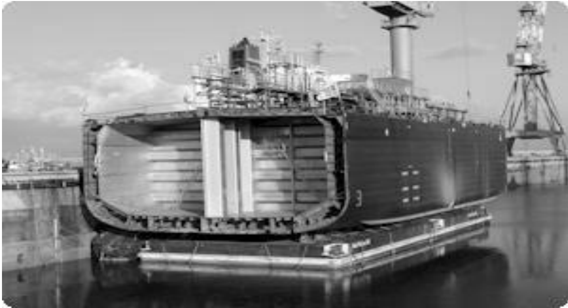
Fig. 1.1 A Sophisticated Parcel Chemical Tanker with Transverse and vertically corrugated Stainless Steel Bulkheads
