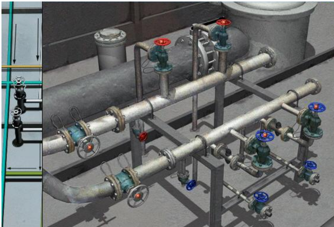
Chemical Simulator Fig1.8H Tank Heating arrangements on a Chemical Tankers main deck
