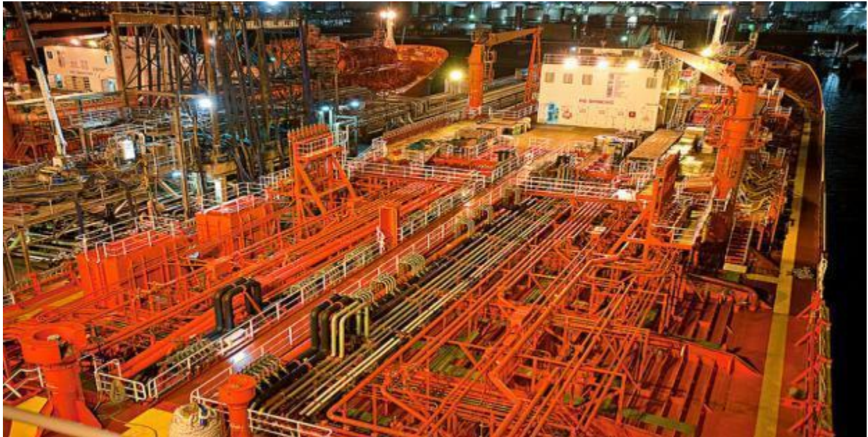
Fig.1.4 A: Chemical tanker Deck pipeline arrangements
