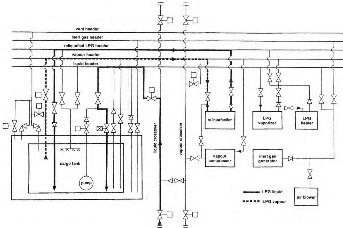
Figure 2.5(F) LOADING, WITHOUT VAPOUR RETURN
