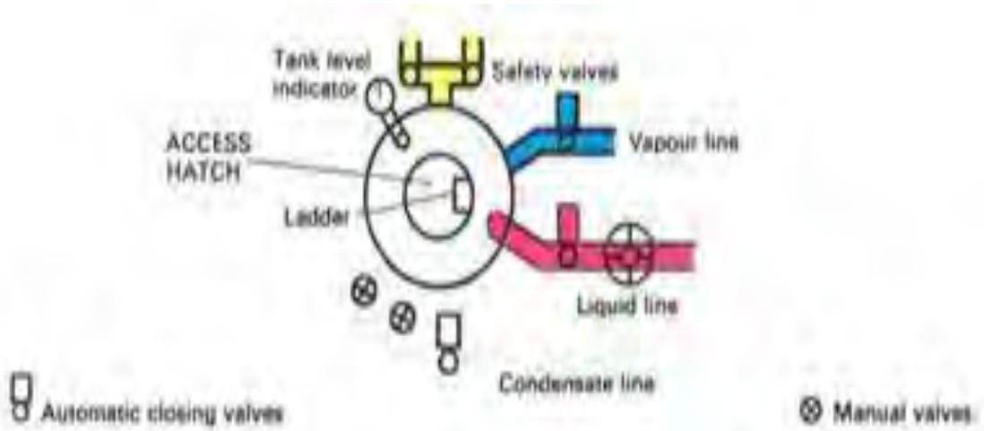
**Figure 1.2 (B) TANK DOME PENETRATION**
