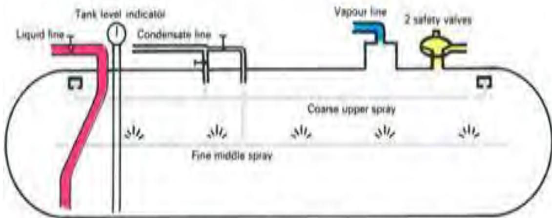
NOTE: An upper cargo tank has been shown for simplicity. In a lower tank, all the piping arrangements enter the tank via the tank dome
