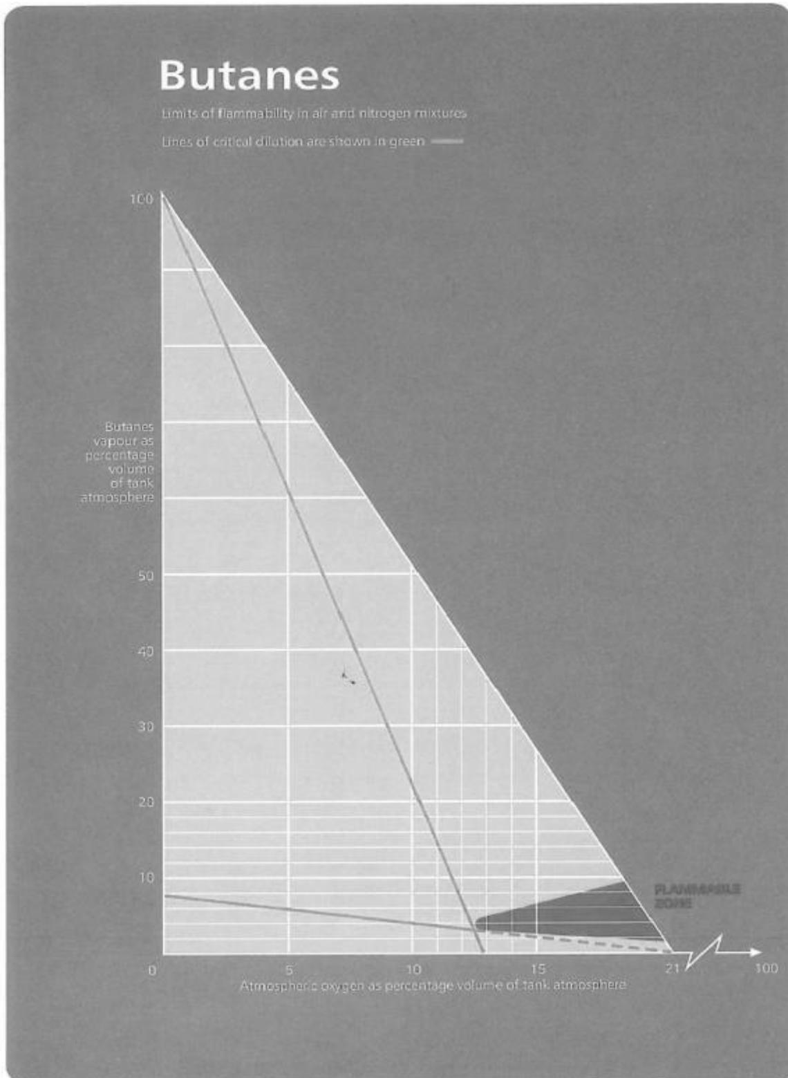
**Figure 6.1.1 FLAMMABILITY DIAGRAM**
