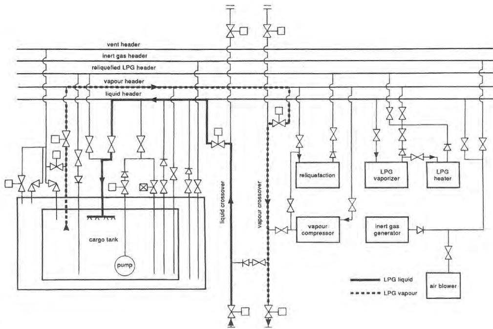
**Figure 2.5(E) COOLING DOWN OF A CARGO TANK, USING LIQUID FROM SHORE AND VAPOUR RETURN**
