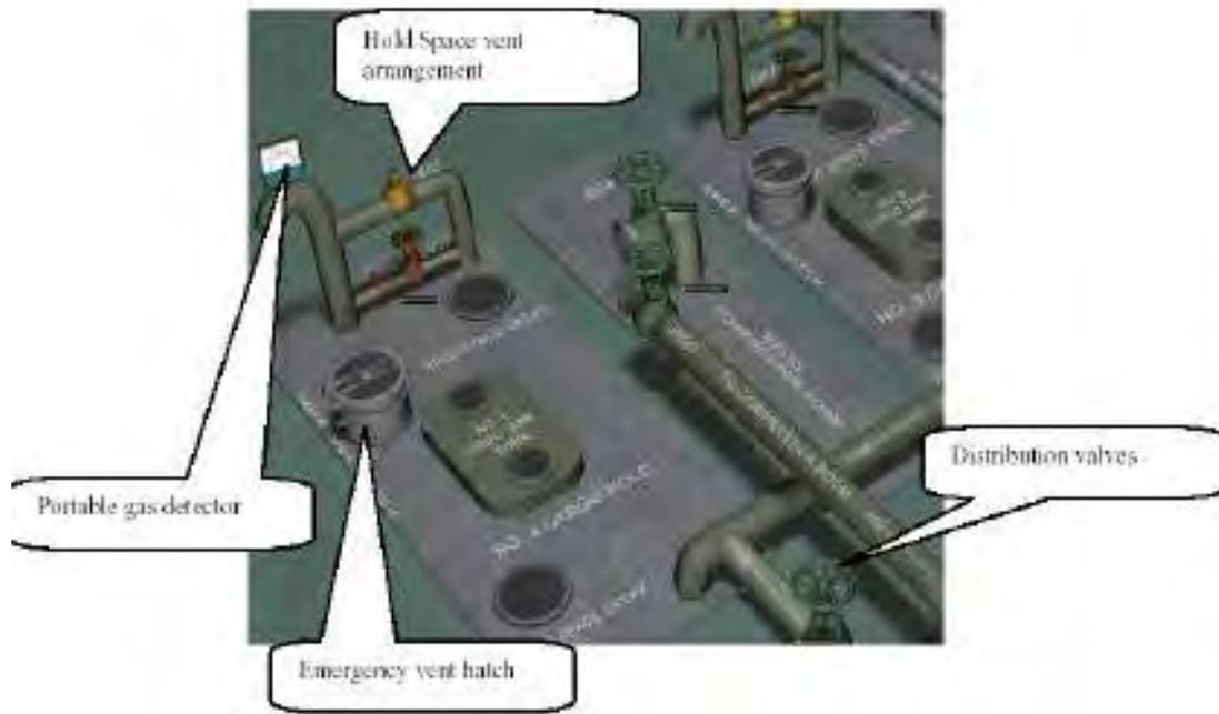
**Figure 2.3.2 (D) INERT / VENTING CONTROL
