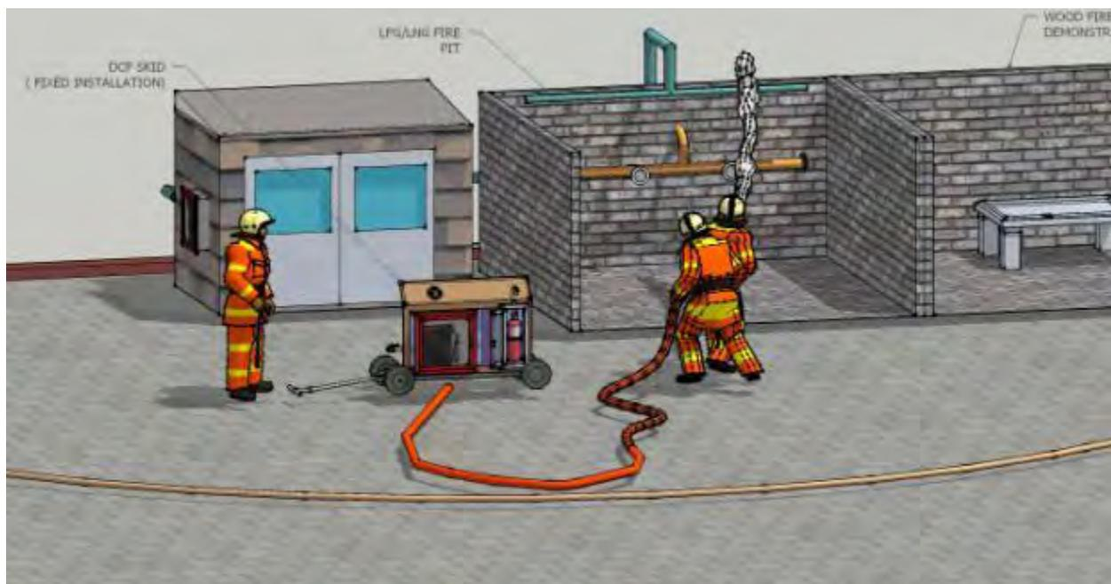
**Figure 2: LPG / LNG fire pit view and demonstration of extinguishing of fire by using fixed DCP system**
