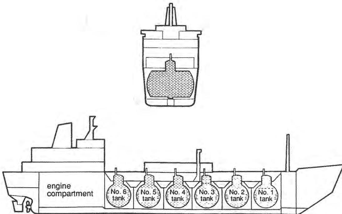
**Figure 1.1 (G) A SEMI – PRESSURIZED FULLY REFRIGERATED LPG / ETHYLENE CARRIER**
