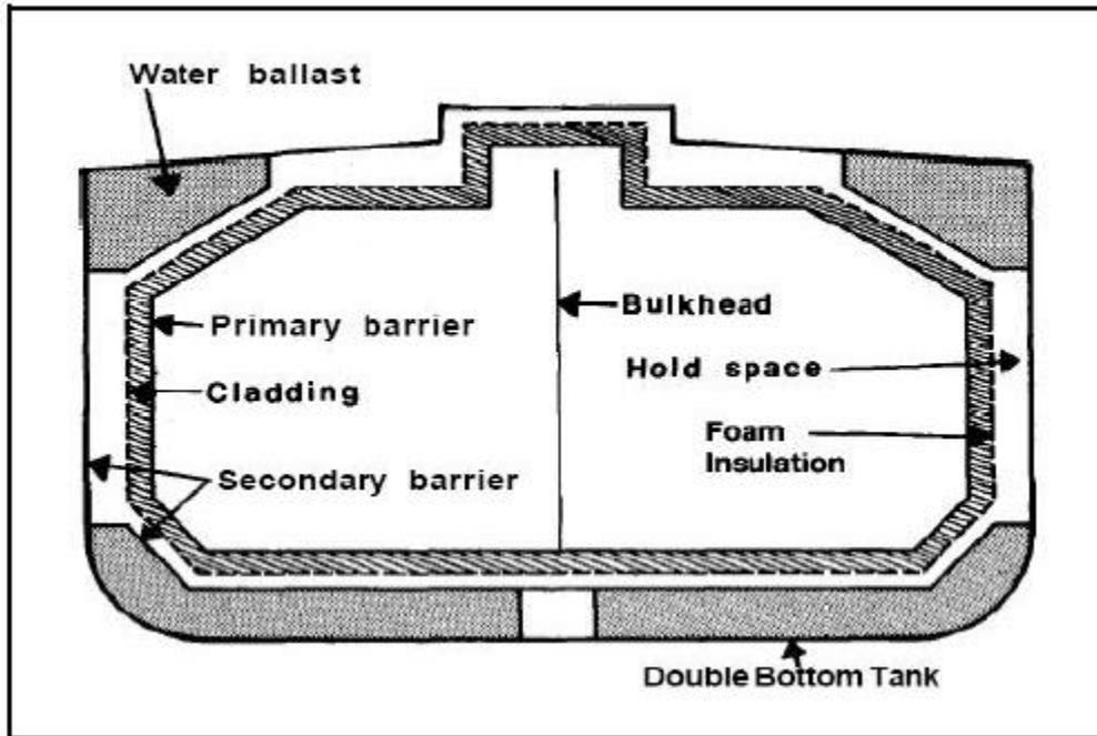
Figure 1.1.8 (A) CONTAINMENT SYSTEM LPG TANK
