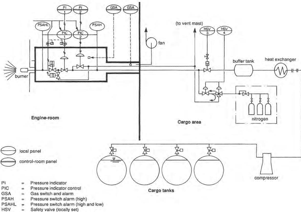
Figure 2.3.2 (C) SCHEMATIC DIAGRAM OF HANDLING OF LNG BOIL-OFF
