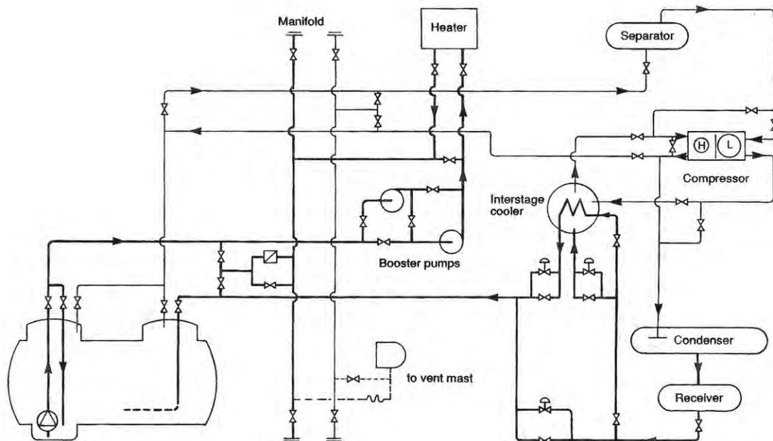
**Figure 2.3(C) CARGO HANDLING ARRANGEMENT LOADING UNLOADING AND CARE IN TRANSIT WITH BOOSTER AND HEATER**
