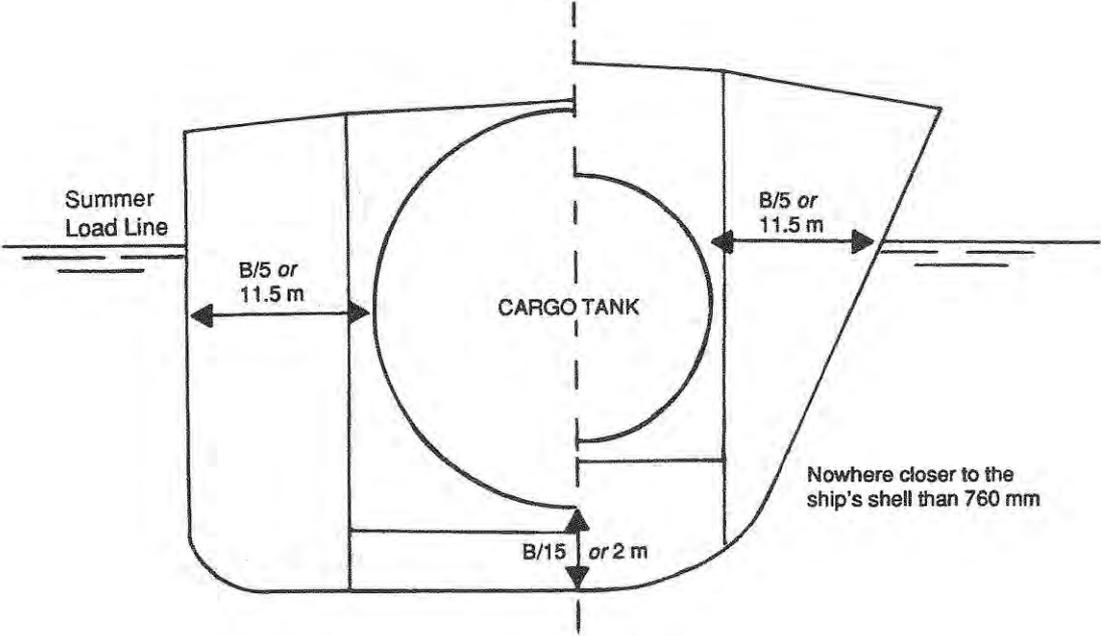
Figure 1.1.8 (I) LOCATION OF CARGO TANKS IN A SHIP OF TYPE 1 G
