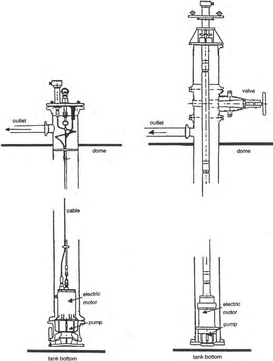
Figure 2.3 (D) EXAMPLES OF ELECTRICAL SUBMERGED PUMPS
