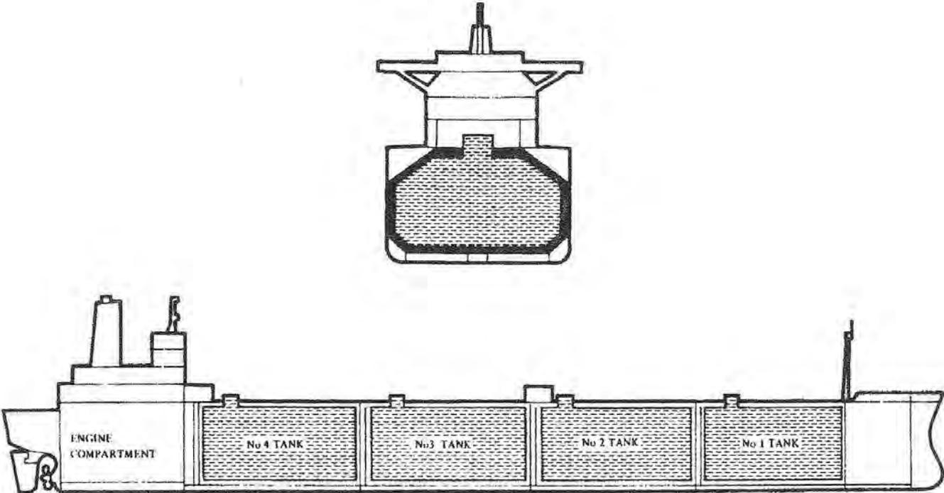
**Figure 1.1 (H) A FULLY REFRIGERATED LPG CARRIER**
