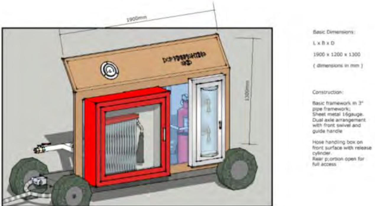
**Figure3: DCP skid front view**
