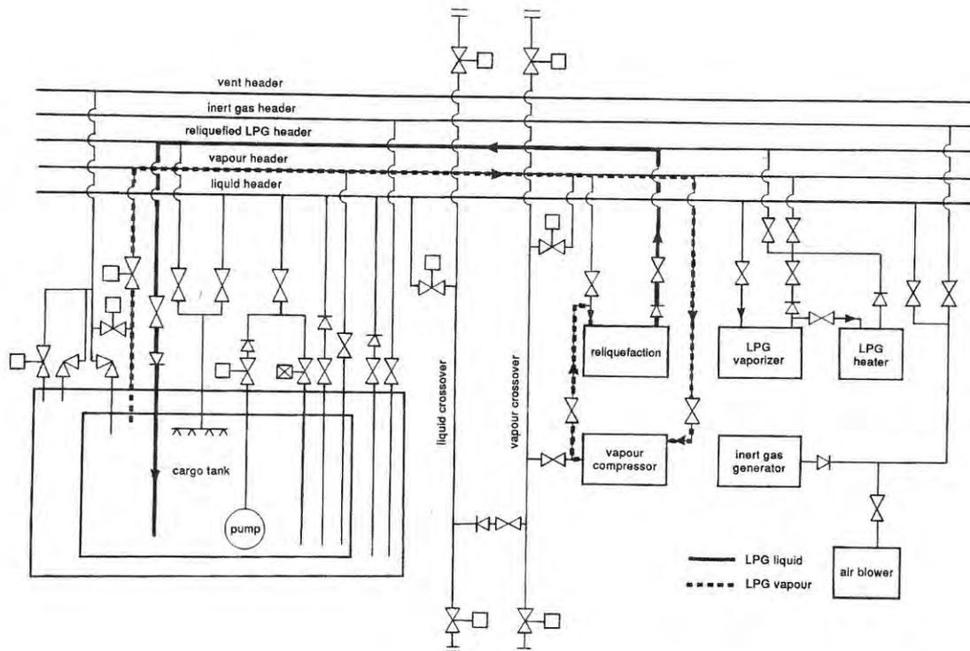
**Figure 2.5(I) CARGO CONDITIONING DURING LOADED PASSAGE**
