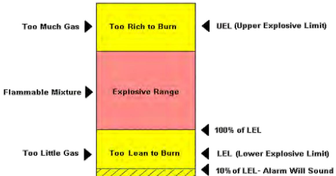
Figure 5.5 (A) FLAMMABLE GAS MIXTURE
