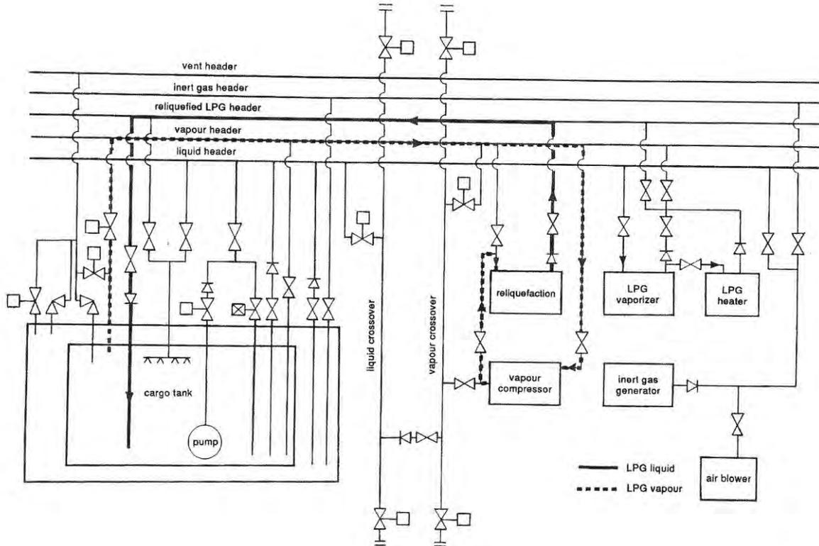
**Figure 2.5(J) CARGO CONDITIONING DURING LOADED PASSAGE**
