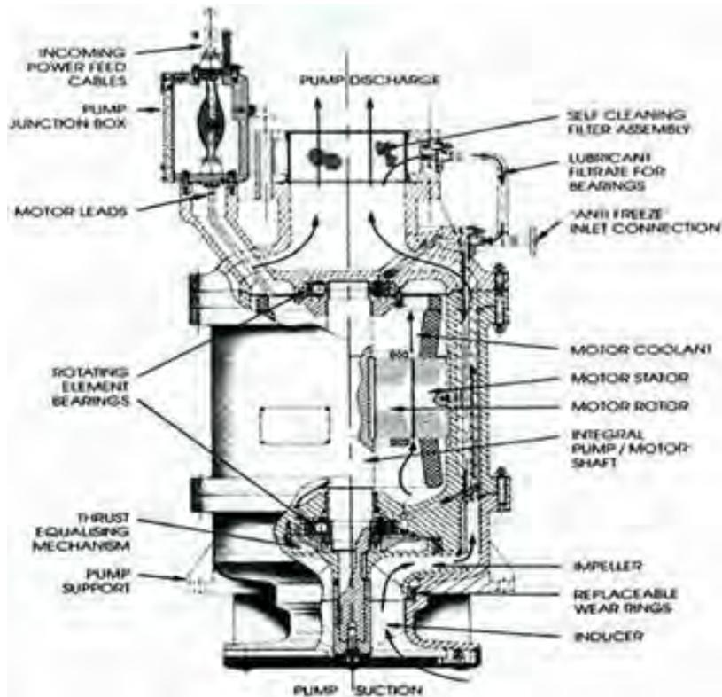
Figure 2.3(I) SUBMERGED MOTOR PUMP FOR LPG
