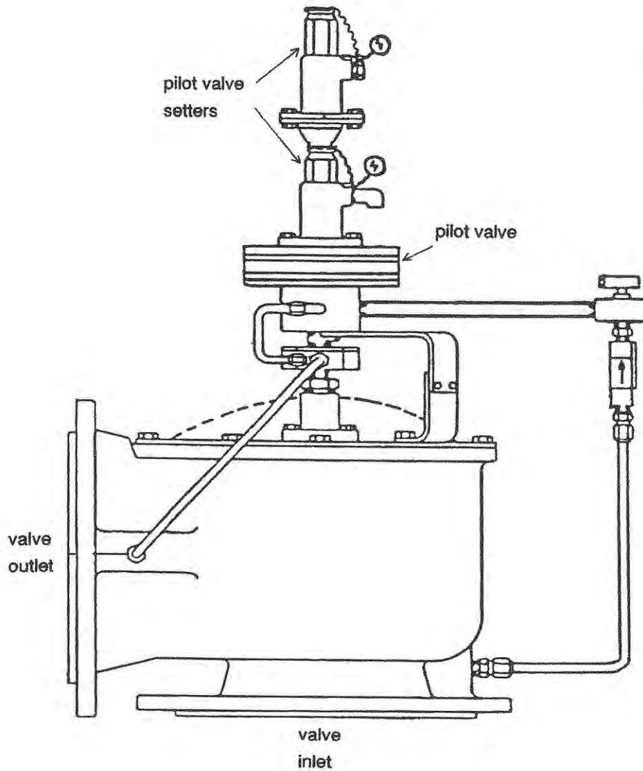
**Figure 2.2.2(A) A CARGO TANK SAFETY RELIEF VALVE**
