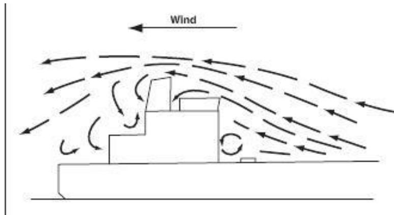
Figure 5.5 (B) FLOW OF EXPLOSIVE VAPOURS IN CASE OF VENTING / LEAKS
