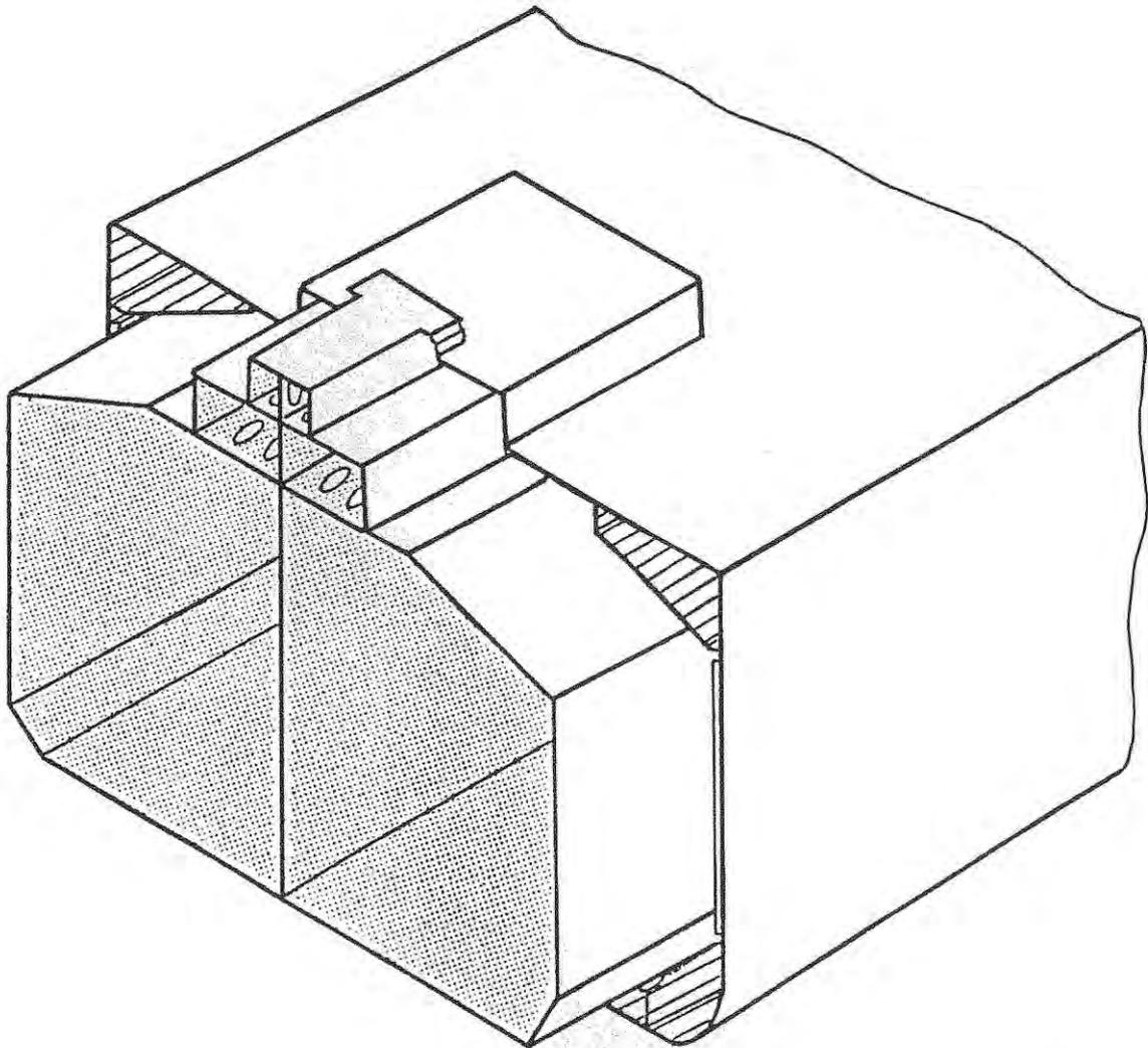
**Figure 1.1.8 (K) AN INDEPENDENT TANK OF TYPE A (FOR LPG)**
