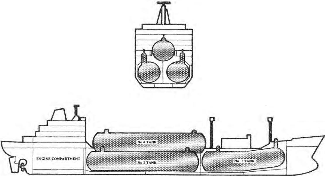
A semi-pressurized/fully refrigerated LPG/NH3 carrier
