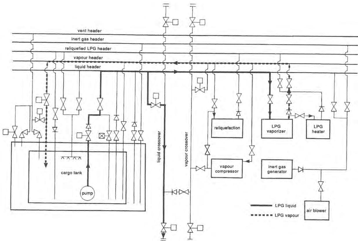
**Figure 2.3 (B) CARGO DISCHARGING, WITHOUT VAPOUR RETURN**
