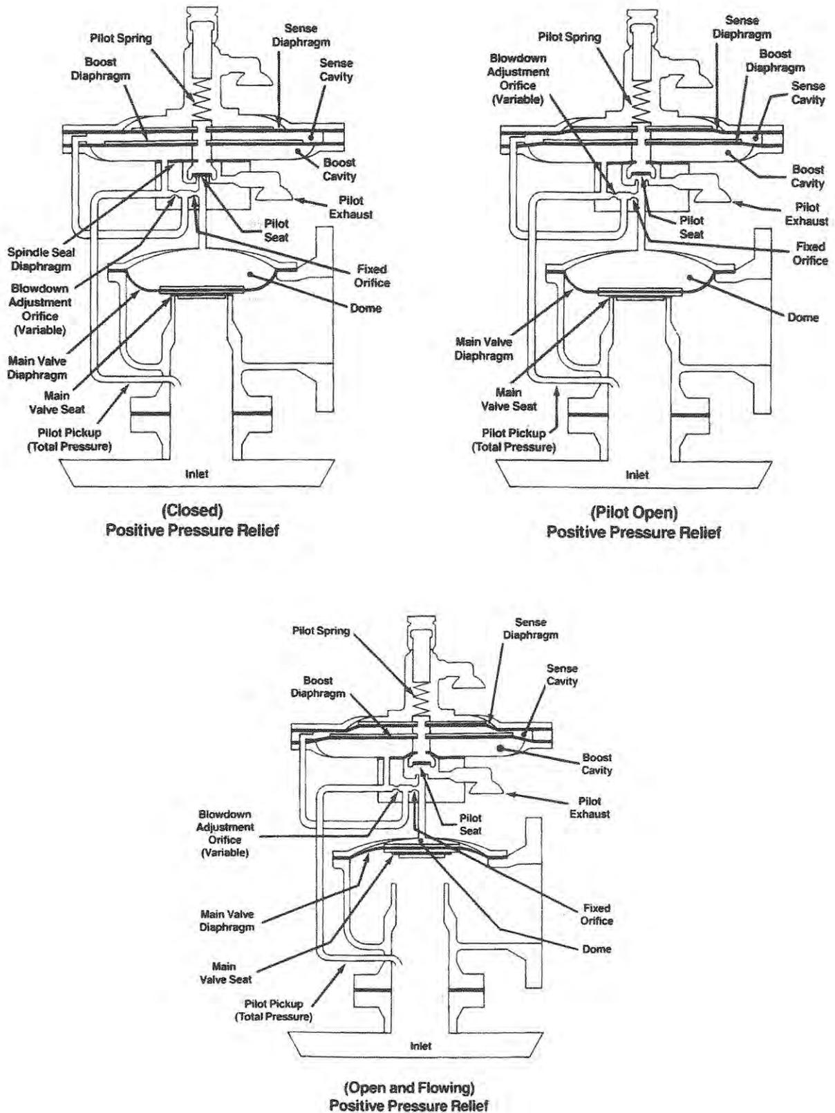
**Figure 2.2.2 (B) OPERATIONAL PRINCIPLE OF A TANK SAFETY RELIEF VALVE**
