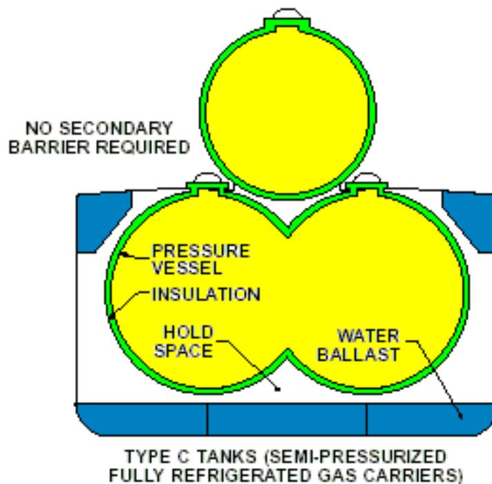
Figure 1.1.8 (D) SEMI PRESSURISED LPG SHIP
