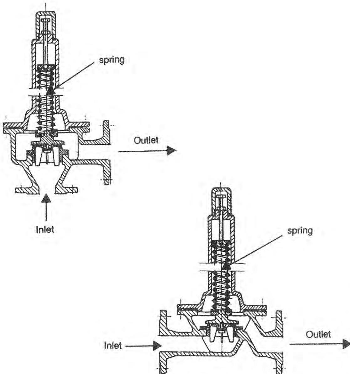
**Figure 2.2.2 (C) SPRING – LOADED RELIEF VALVES**
