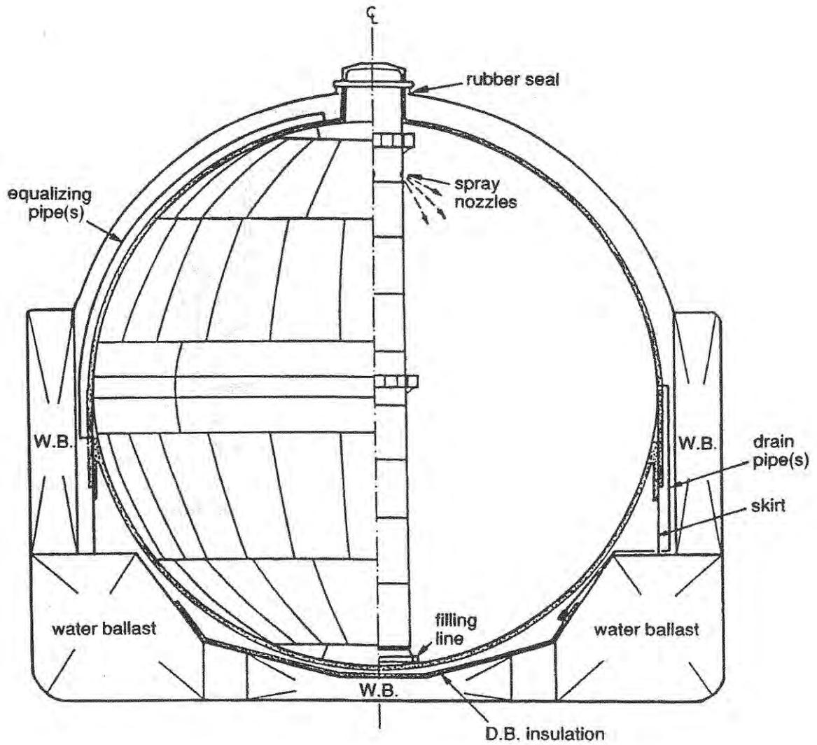
**Figure 1.1.8 (H) AN INDEPENDENT TANK OF TYPE B**
