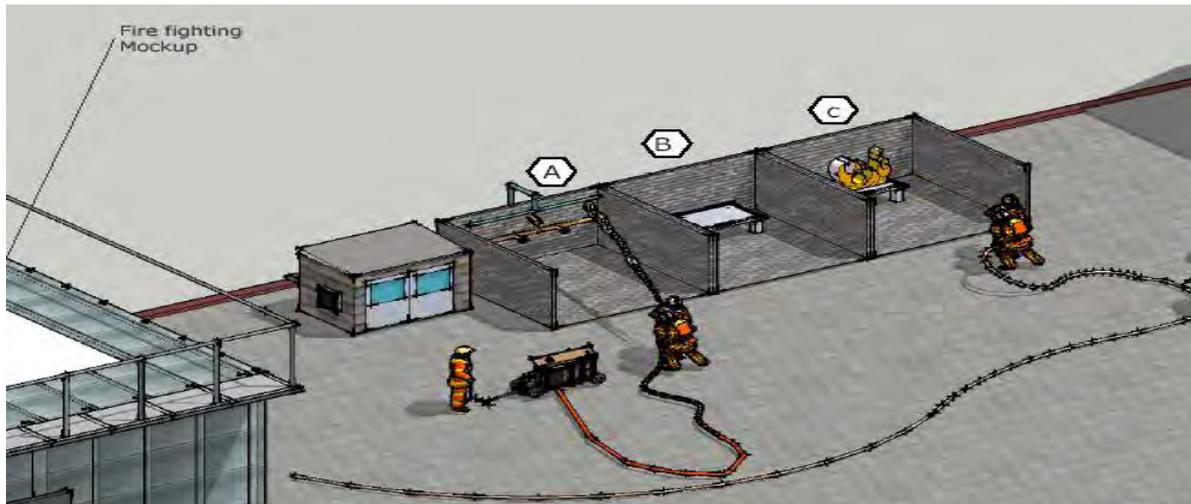
Section A, B and C for Gas, Wood and Oil fire demonstration
