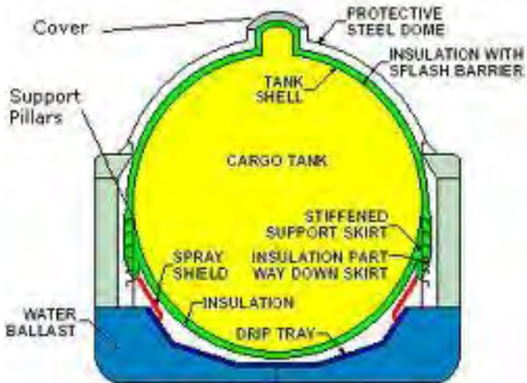
Figure 1.1.8 (E) SELF-SUPPORTING SPHERICAL TYPE B TANK
