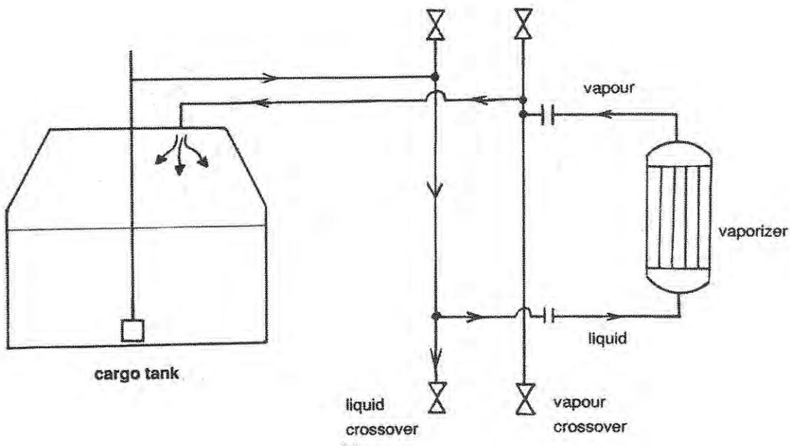
Figure 2.2.3(B) SCHEMATIC DIAGRAM OF A VAPORIZER ARRANGEMENT
