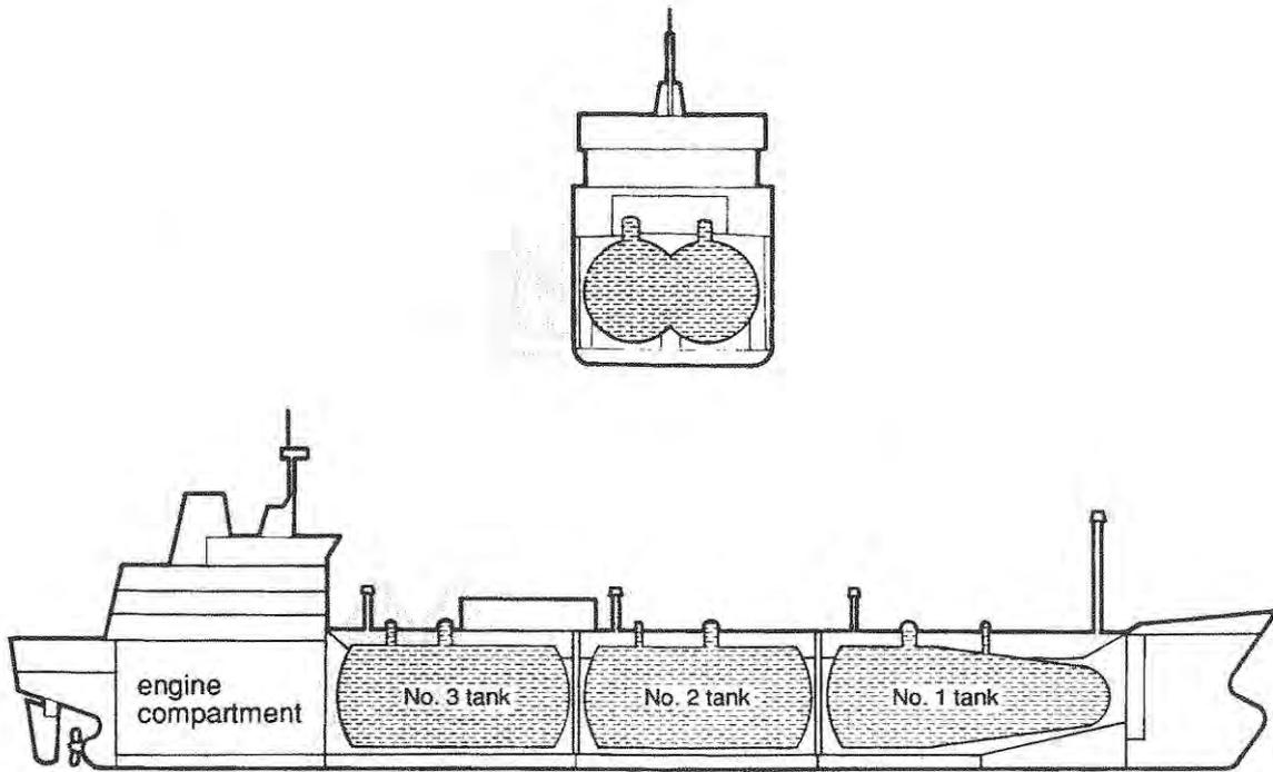
A semi-pressurized/fully refrigerated LPG/NH<sub>3</sub> carrier
