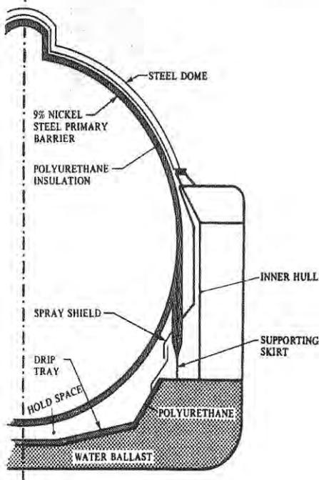
Independent self-supporting spherical tank (type B)
