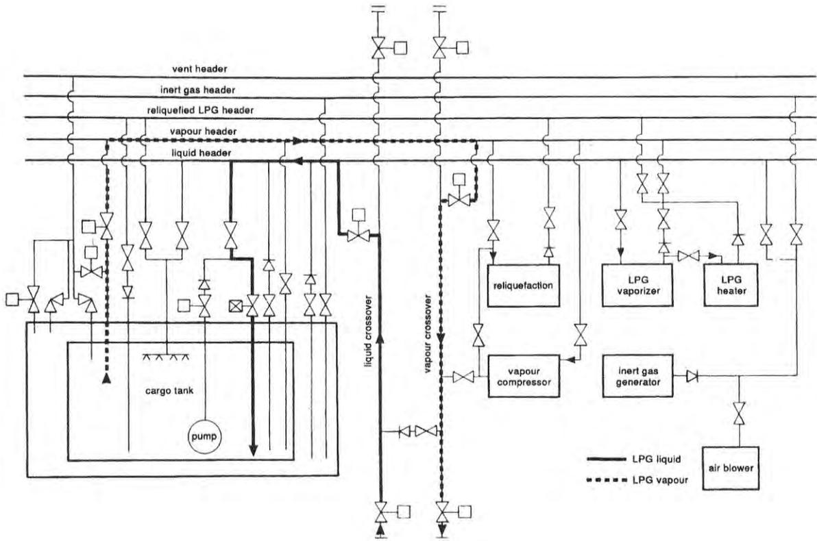
Figure 2.5(G) LOADING, WITH VAPOUR RETURN
