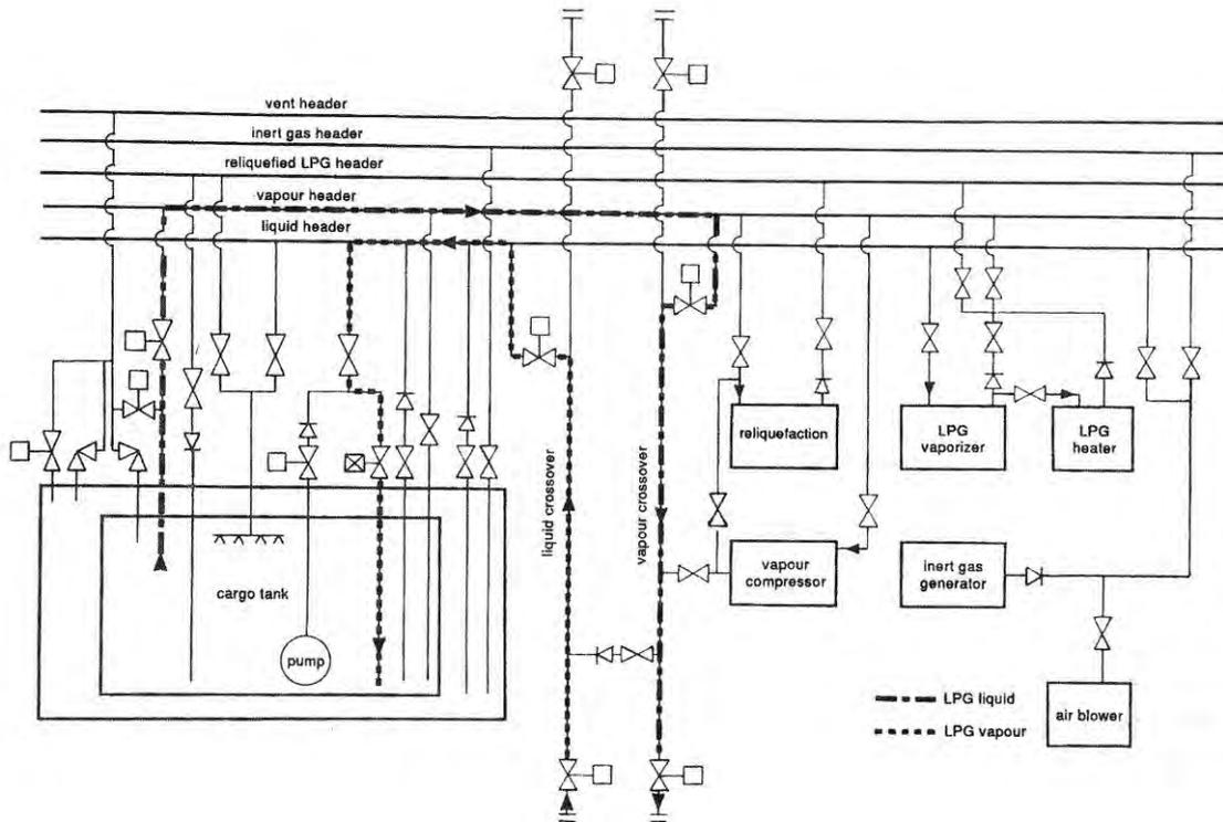
**Figure 2.5(D) PURGING OF A CARGO TANK, USING VAPOUR FROM SHORE**
