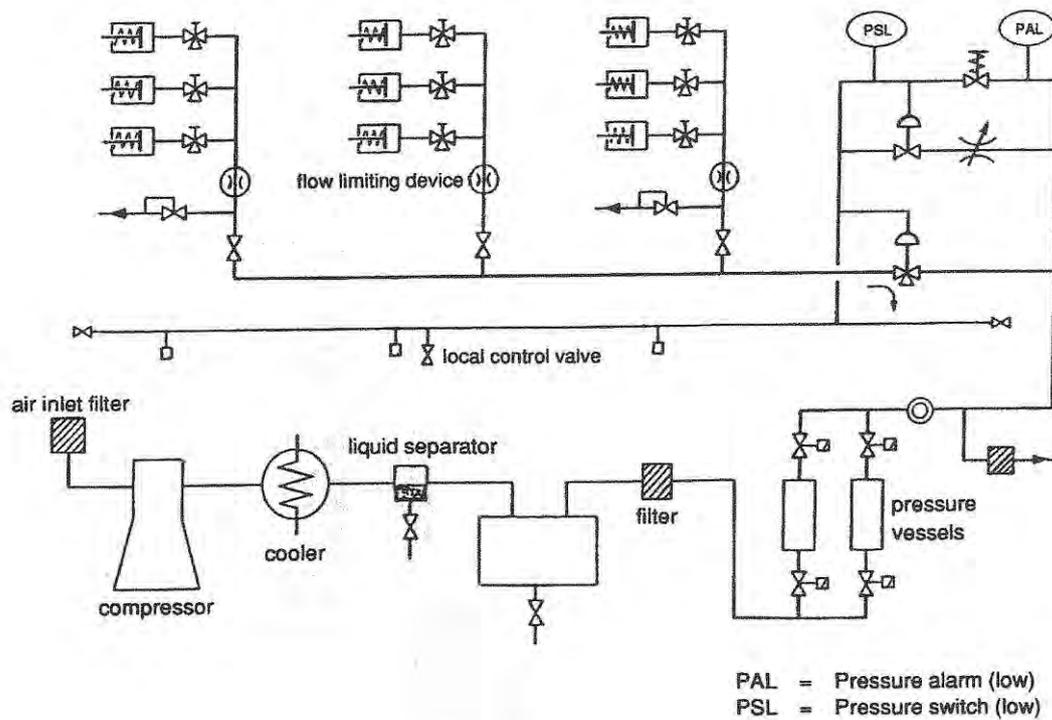
Figure 2.4(B) A PNEUMATIC EMERGENCY SHUTDOWN SYSTEM
