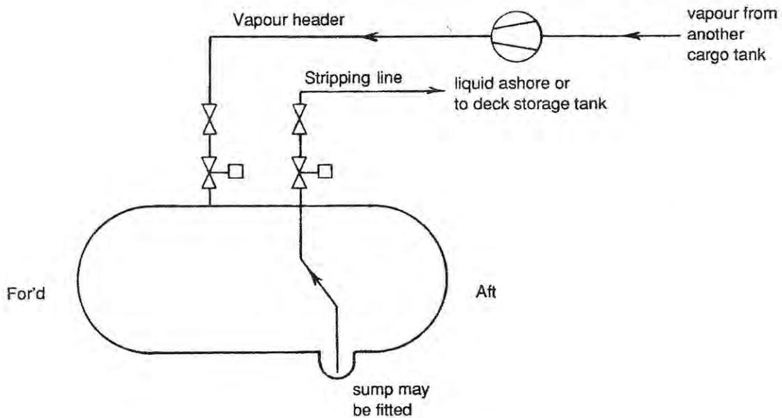
**Figure 2.1.10 REMOVAL OF RESIDUAL CARGO LIQUID BY PRESSURIZATION**
