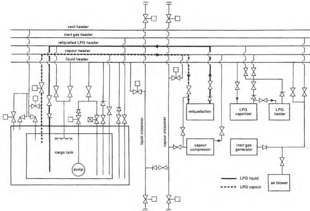
**Figure 2.5(H) COOLING DOWN OF TANKS DURING LOADED PASSAGE**
