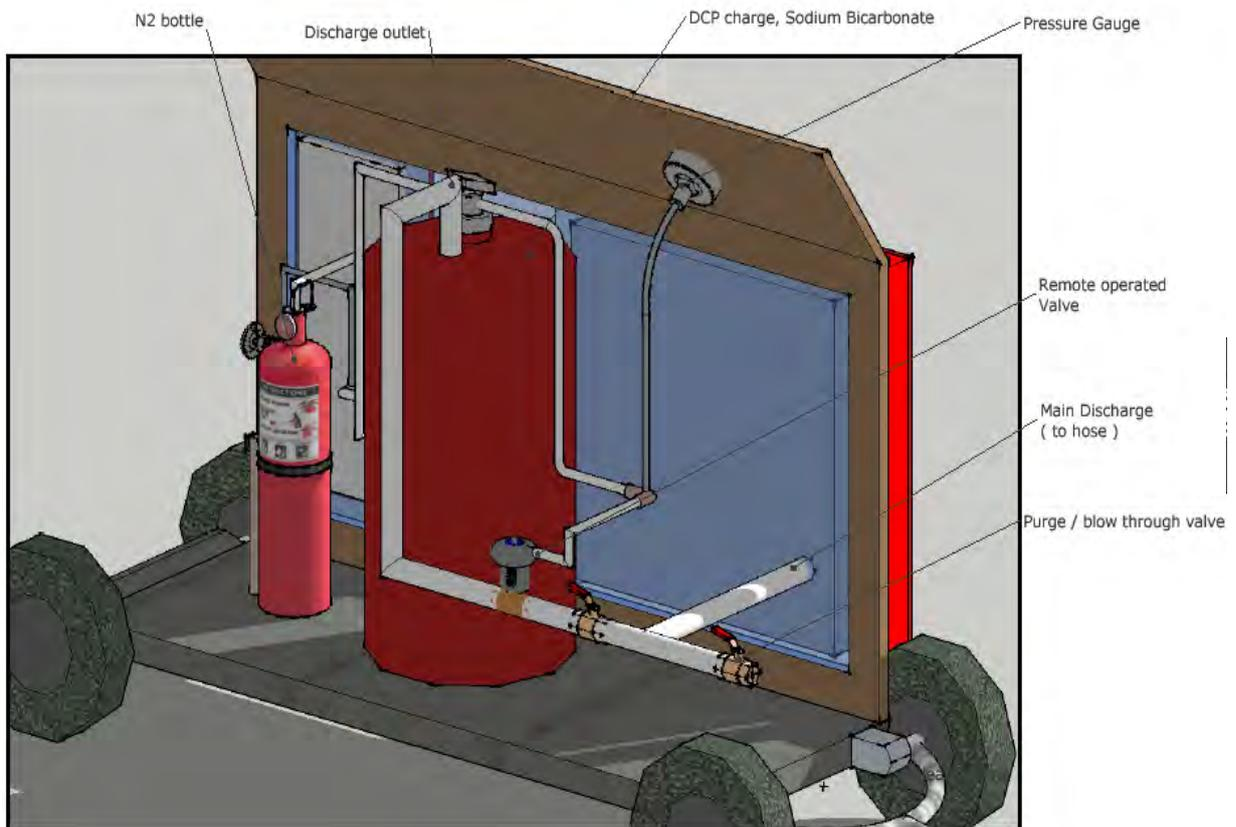
**Figure 4: DCP skid (rear view)**
