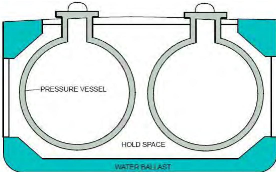
Figure 1.1.8 (B) FULLY PRESSURED CONTAINMENT SYSTEM
