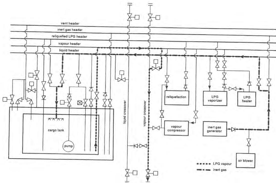
**Figure 2.5 (C) INERTING/PURGING OPERATION**
