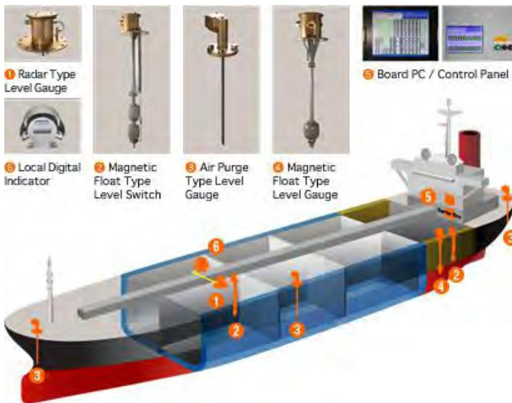
Figure 2.2.1.4 CARGO HANDLING EQUIPMENT- GAUGES
