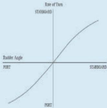
Relation between Rudder Angle and Yaw (Turn) Rate for Straight-line Stable Vessel
