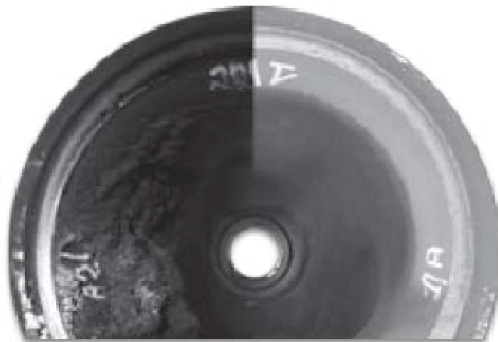
comparison of slide fuel valve before and after retrofitting
