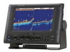
It operates with the principle of sound waves from the bottom of the ship and then measuring the time required for the return of the echo from the sea. If the speed of sound in water is known, time will be proportional to the distance travelled.
