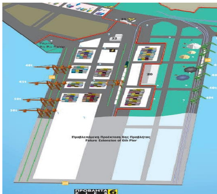
Photo 2.3 Future extension of 6 th Pier. [Available: http://www.thpa.gr/files/general/thpa_4p_en.pdf (accessed on 24th September 2014)].
