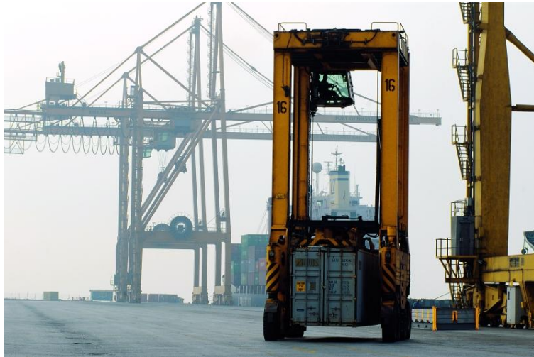
Photo 2.1 Straddle carrier at the port of Thessaloniki. [Available: http://www.thpa.gr/images/sempo/ct01.jpg (accessed 28 th July 2014)].
