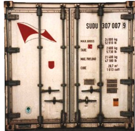
Picture 2.3.4.1: Marking on the door of a container
