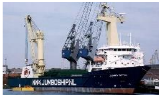
EIKONA 6 VESSEL HAVING A COMBINATION OF CRANEDERRICKS
