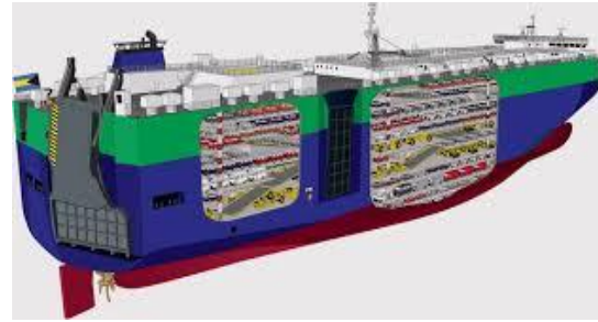
EIKONA 15 THE INSIDE OF A RO-RO VESSEL
