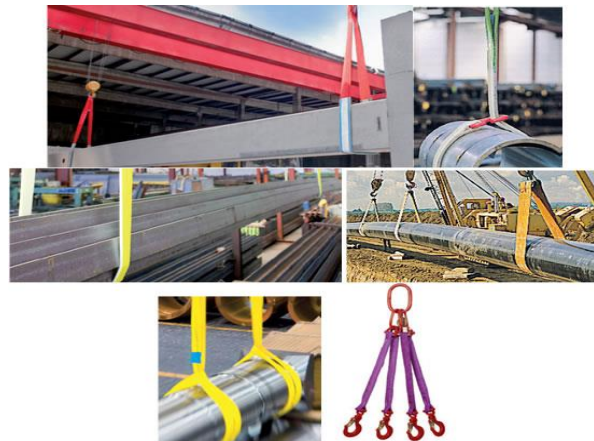
EIKONA 11 DISCHARGING OPERATION THROUGH ENDLESS BELTS
