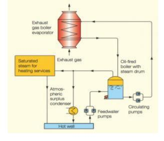
An Exhaust Gas Boiler is a type of heat recovering system on ships which allows the exhaust heat of the main engine to produce steam while going out in the atmosphere.
