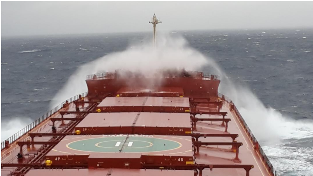
Picture 5.4 Bulk carrier , deck wetness due to high waves
