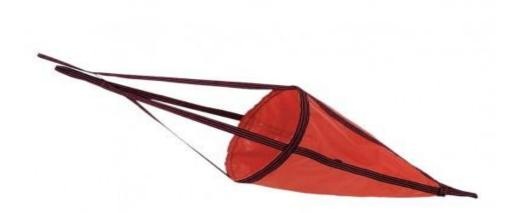
You make this adjustment by opening or closing the sea anchor's apex. When open, the sea anchor acts as a drag that keeps you in the general area. When closed, it forms a pocket for the current to strike and propels the raft in the current's direction. Additionally, adjust the sea anchor so that when the raft is on the wave's crest, the sea anchor is in the wave's trough. Wrap the sea anchor rope with cloth to prevent its chafing the raft.
