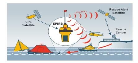
If possible, the EPIRB should be recovered and tied (using its lanyard) to one of the liferafts. An EPIRB is meant to mark survivors, not he accident scene. For best operation leave the EPIRB floating in the sea near the liferaft. If your EPIRB has been activated for a cumulative period in excess of 2 hours then its battery will need replacing. This is necessary to ensure that the next time it gets used it will operate for the full 48 hours required by government regulations.
