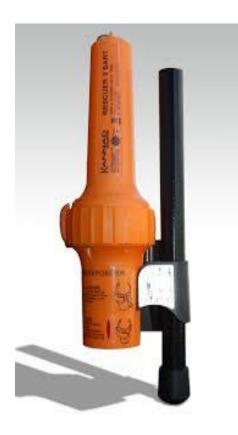
The bright color of SARTs enables their quick detection, whereas the combination of transmitter and receiver enables it to transmit as well as receive radio signals. SART machines have been instrumental in rescuing several crafts and ships by reacting to the search signal sent from an X-band radar, typically of 9 GHz. These signals are known as homing signals.
