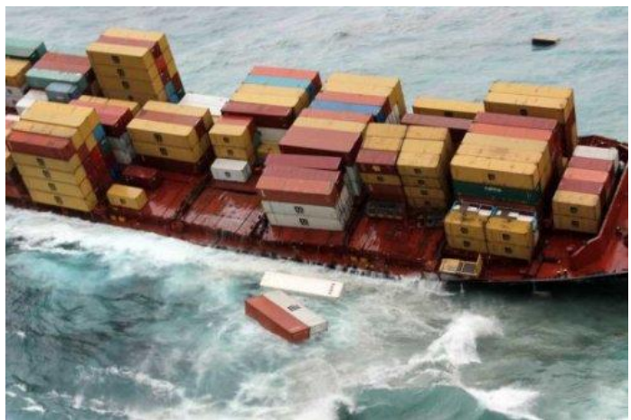
Picture 2.3.1 Loss of stability due to mistaken stowage
