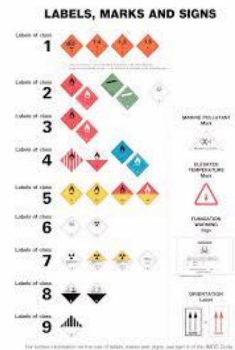
Picture 2.2.1 Labels, marks and signs
