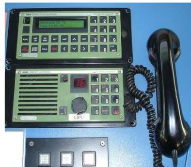
Marine VHF radio equipment is installed on all large ships and most seagoing small craft. It is also used, with slightly different regulation, on rivers and lakes. It is used for a wide variety of purposes, including summoning rescue services and communicating with harbors, locks, bridges and marinas.
