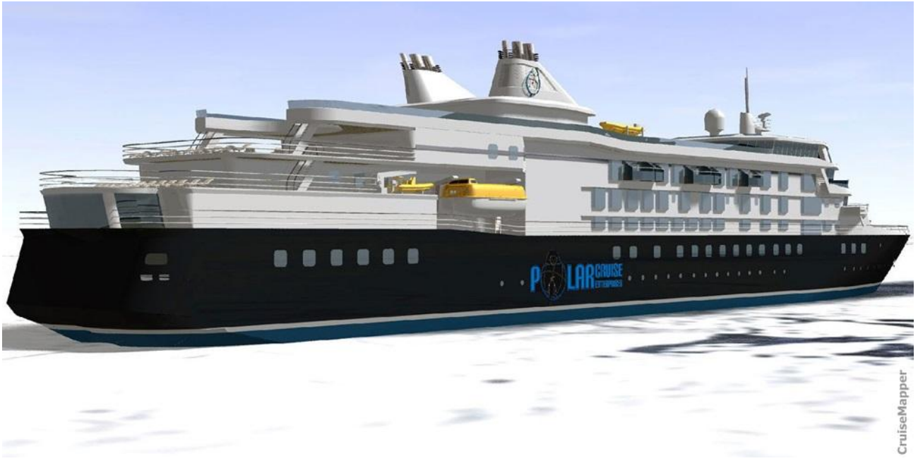
Knud E Hansen's expedition ship design with 150 cabins and heavy-duty, ice-rated hull. ( http://www.cruisemapper.com/wiki/757-cruise-ship-building-construction-design )
