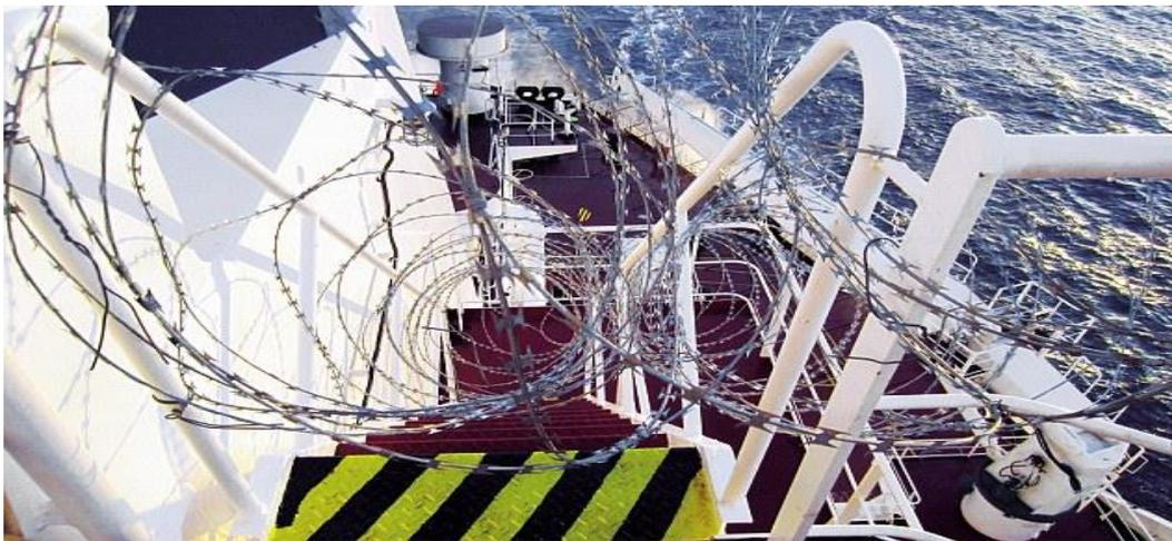
Razor wire (also known as barbed tape) creates an effective barrier but only when carefully deployed. The barbs on the wire are designed to have a piercing and gripping action. Care should be taken when selecting appropriate razor wire as the quality (wire gauge and frequency of barbs) and type will vary considerably. Lower quality razor wire is unlikely to be effective. Three main types of razor wire are commonly available:
