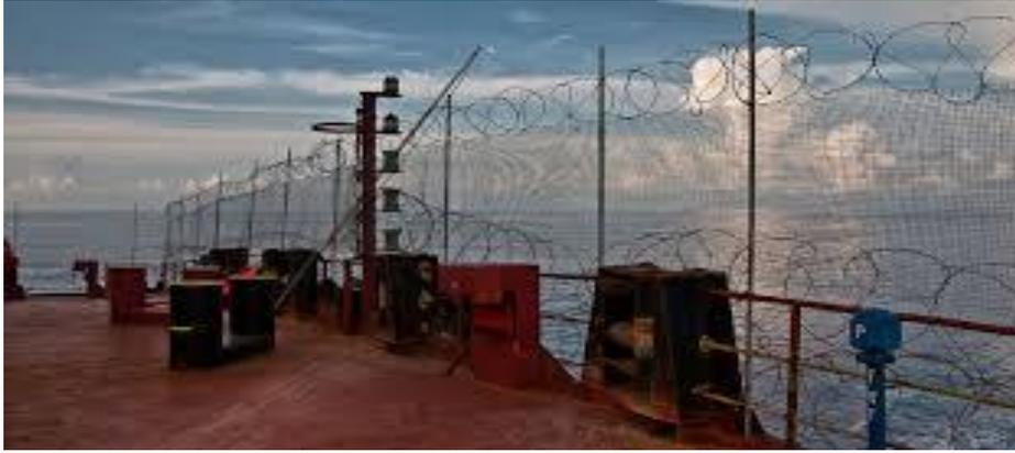
Electrified barriers are not recommended for hydrocarbon carrying vessels but, following a full risk assessment, can be appropriate and effective for some other types of vessel. It is recommended that warning signs of the electrified fence or barrier are displayed - inward facing in English/language of the crew, outward facing in Somali. The use of such outward facing warning signs might also be considered as a deterrent even if no part of the barrier is actually electrified
