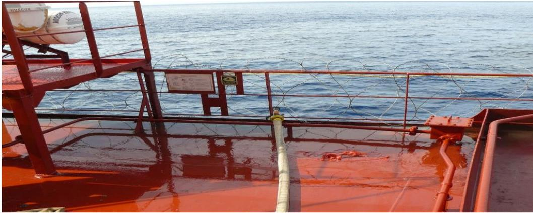
Water cannons – These are designed to deliver water in a vertical sweeping arc thus protecting a greater part of the hull. Many of these have been developed from tank cleaning machines.
