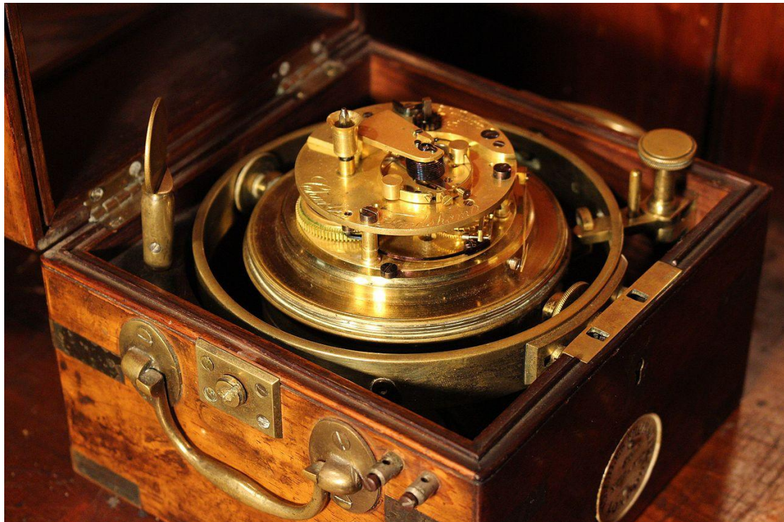
A marine chronometer by Charles Frodsham of London, shown turned upside down to reveal the movement. Chronometer circa 1844-1860.
