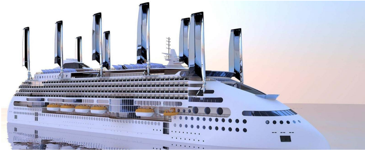
Figure 2: Peace Boat Ecoship, ice class Type C vessel with wind energy system https://www.google.gr/imghp?hl=el&tab=wi&ogbl
