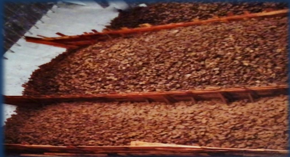
Pic.28 General & Break-Bulk Cargoes (Separation fences for pig iron)
