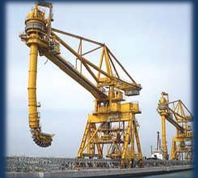
Pic.9 Continuous Ship Unloader and Loader
