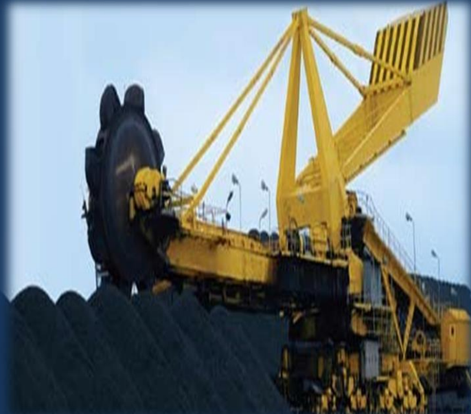
Pic.11 Stockyard Reclaimer Crane
