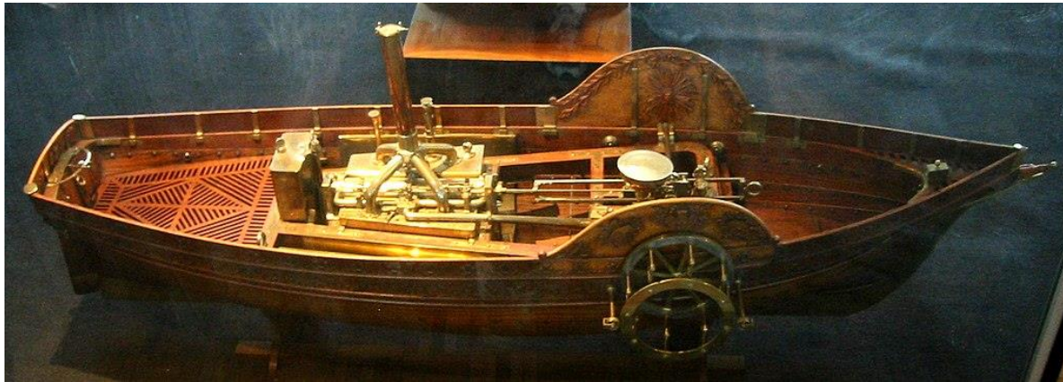
Model made by Jouffroy in 1784 to show the French Science Academy the engine and paddle wheels used on the Pyroscaphe. The model is now in the National Maritime Museum in Paris.
