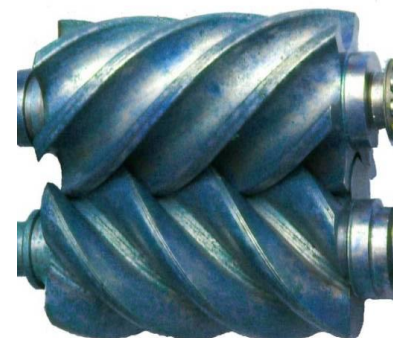
Lysholm screw rotor
