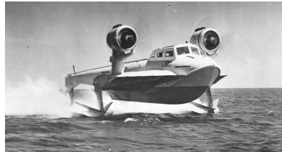
The US Navy's XCH-4, with hydrofoils clearly lifting the hull out of the water
