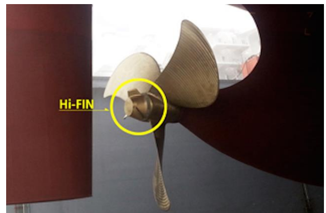
Hi-FIN attached to a ship's propeller
