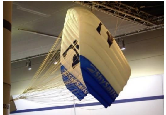
A prototype kite (production kites have areas of hundreds of square meters)
