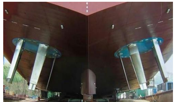
Ship fitted with a Voith Schneider Propeller
