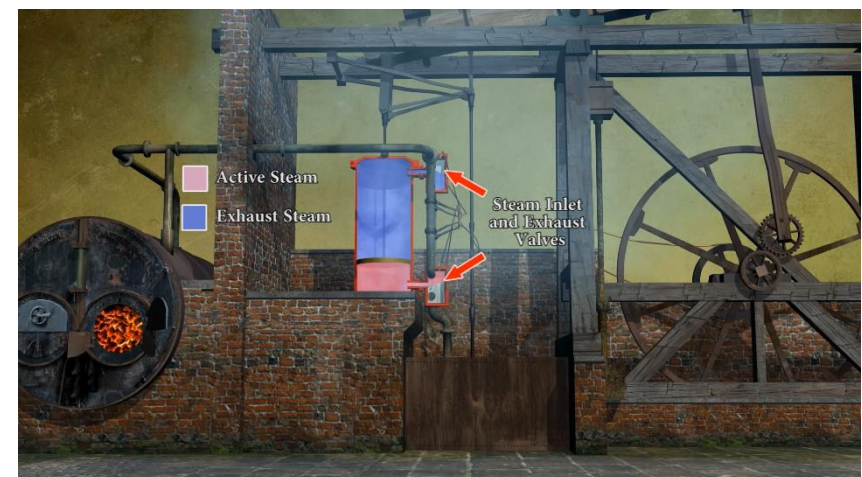
Bottom - Equilibrium valve open at end of the down-stroke
