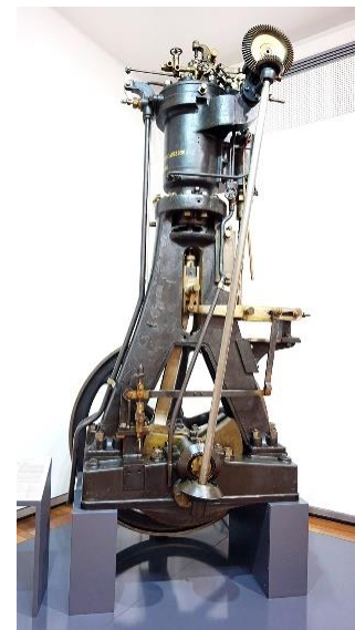
Diesel's second prototype. It is a modification of the first experimental engine. On 17 February 1894, this engine ran under its own power for the first time
