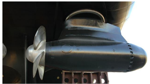
Closeup of one of USCGC Mackinaw's 3.3 MW Azipod units
