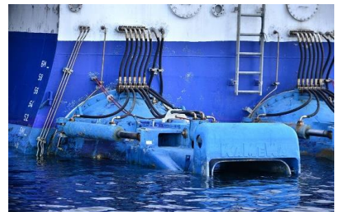
Two of four KaMeWa waterjets on the high-speed ferry Discovery
