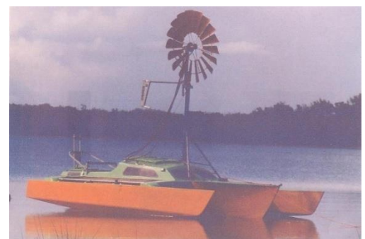
"Thrippence" Windmill Catamaran with a 6-foot-tall mill
