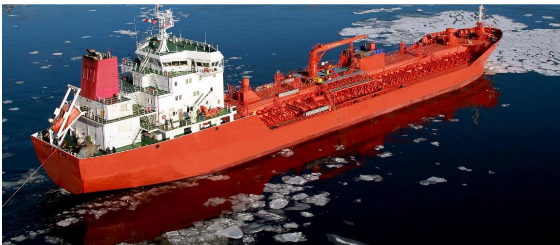
Picture 1.3.: Chemical tanker transporting noxious liquid substances in bulk.
