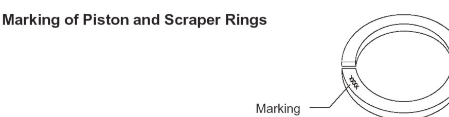
Identification marks to face upwards against the piston crown when mounted.
