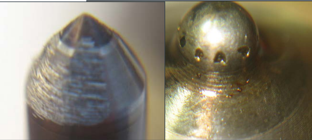
Damage due to cat fines
