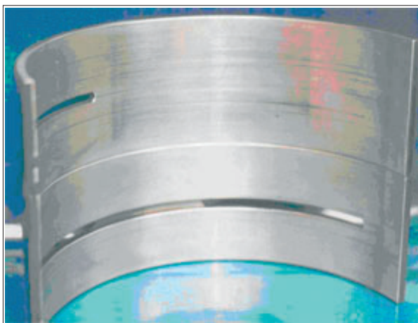
Fig 3 Acceptable level of contaminant. Can refit.
