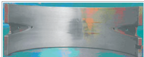
Fig 2 A104 bearing after 22,000 hours. Can refit.
