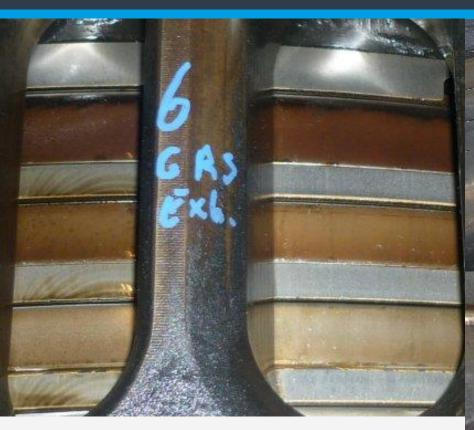
Ex. CMA CGM Debussy, 12K98MC-C. GRS test liner with 6490 hours
